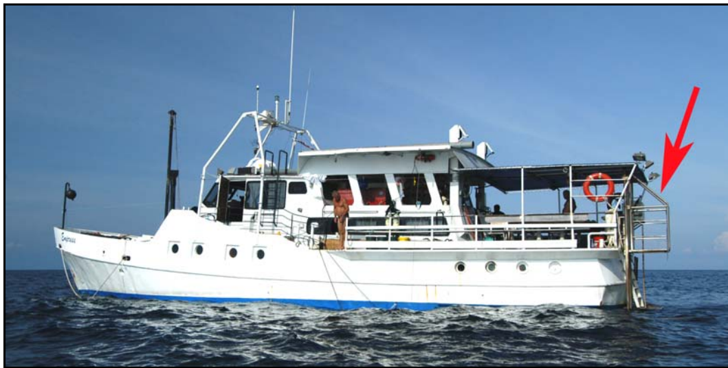
MV Empress. Note divers lift, or elevator, at stern (red arrow). When this is lowered into the water a heavily laden diver simply swims into the 'cage', stands up and is lifted back on board. Sure beats climbing up a dive ladder!
