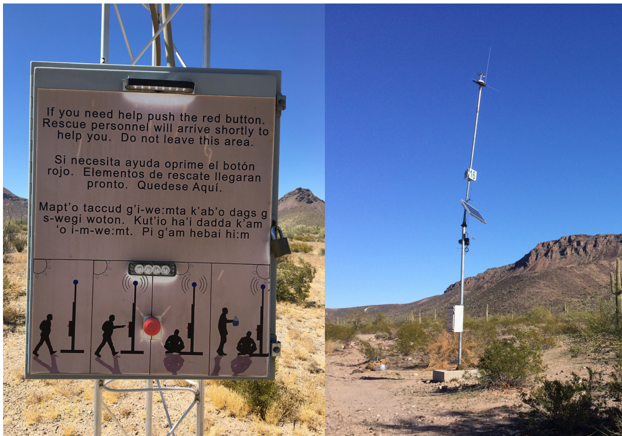
Border Patrol beacons are metal towers ranging from 20 to 40 feet high with a blue-strobe LED light affixed at the top. The beacons have a large red button on them; some are equipped with a satellite phone. 115
