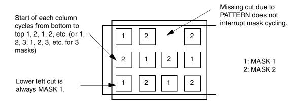
Assuming that the layer VIA1 is a two-mask cut-layer, then the mask color for each cut-shape is a checker-board as shown above. The default checker-board pattern is: the bottom left cut starts at 1, and then goes from left to right, 1, 2, 1, 2. The next row starts at 2, and goes 2, 1, 2, 1, etc. The missing cuts due to PATTERN statement do not change the mask assignments.
