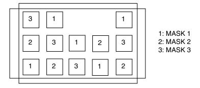
Example of a parameterized via checker-board cut-mask pattern for a 3-mask layer with 2 missing cuts. For parameterized vias (with VIARULE . . . ), the mask of the cuts are pre-defined as an alternating pattern starting with MASK 1 at the bottom left. The mask cycles from left-to-right and bottom-to-top are shown.
