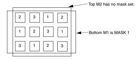
Masks for via-instance: VIA MASK 031 15 15 VIA1\_2; Bottom M1 is MASK 1. Top M2 has no mask set. Lower-left cut is MASK 3, and other via-instance cut shape masks are derived from via-master cut-masks as shown above by "shifting" the via-master masks to match: 1->3, 2->1, 3->2.
