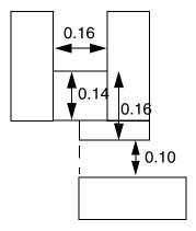
d) Okay. Notch metal width is >= 0.15 for the overlap; therefore extra space is not required.
