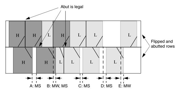
MS = Minimum spacing error MW = Minimum width error
