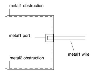
Routing can also connect to such a port on the same layer if the routing does not cross any obstruction by more than a distance of the total of minimum width plus minimum spacing before reaching the pin. This is because the port geometry is known to be "real," and any obstruction less than a distance of minimum width plus minimum spacing away from the port is not a real obstruction. If the pin is more than minimum width plus minimum spacing away
