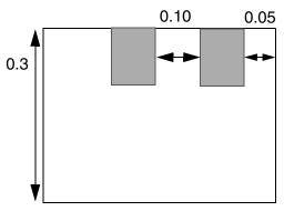
d) Okay; extra cut is <= 0.2 away; therefore, use min-width rule, and both cuts meet min-width enclosure rule of 0.0 and 0.5.
