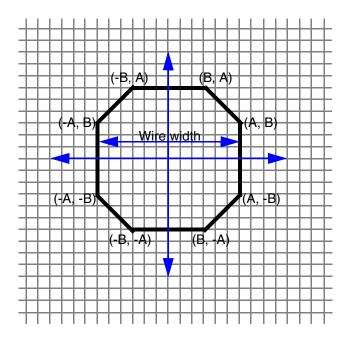
The octagon is always symmetric about the x and y axis. The coordinates are computed to be exactly the same wire width as equivalent horizontal or vertical wire widths, and as close as possible for the diagonal widths (they are always slightly bigger because of rounding of irrational values), while forcing the coordinates to remain on the manufacturing grid. The wire width must be an even multiple of the manufacturing grid in order to keep A and B on the manufacturing grid.
