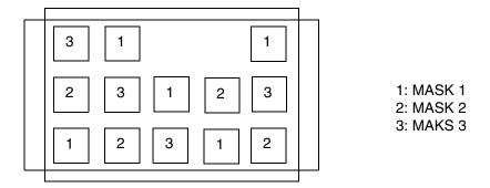
Example of a check-board parameterized via cut-mask pattern for a 3-mask layer with 2 missing cuts due to PATTERN statement.
