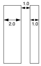
a) Okay if both wires are the same net and are either a power or ground net.
