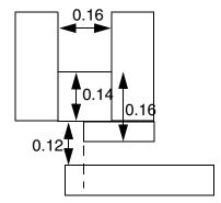
e) Violation. Notch metal width is < 0.15 for part of the overlap; therefore 0.14 spacing is required.
