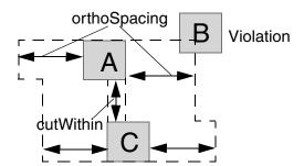
d) The rule applies in both the X and Y directions. In this case, the horizontal overlap of A and C makes B a violation.
