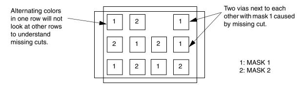
Unlike parameterized vias, there is no real row/column structure required in a fixed via, so the automatic coloring will not work well for a fixed via with missing cuts (or cuts that are not aligned). This type of via must be pre-colored to be useful.
