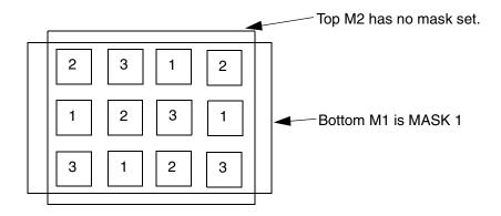
Masks for via-instance: ... ( 20 20 ) MASK 031 VIA1\_2; Bottom M1 is MASK 1.Top M2 has no mask set. Lower-left cut is MASK 3, and other via-instance cut shape masks are derived from via-master cut-masks as shown above by "shifting" the via-master masks to match: 1->3, 2->1, 3->2.
