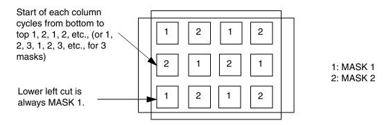
Uncolored fixed vias (from RECT/POLYGON statements) will get similar coloring as a parameterized via. Each cut with the same Y value is one row. The cuts inside one row alternate. This works well for cut-arrays without missing cuts as shown above.
