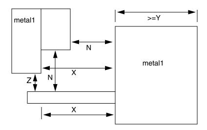
In the following example, the 0.5  $\mu$ m spacing applies for the first 1.0  $\mu$ m of the stub sticking out from the large object. This rule only applies to the stub wire; the previous rule must be included for the wide wire spacing. The SPACING 0.5 RANGE 2.01 2000.0 statement is required to get extra spacing for the wide-wire itself.
