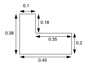
b) OK, the 0.18 vertical segment does not count as the wrong direction width. The wrong direction width along that edge is actually 0.2 + 0.18 = 0.38.
