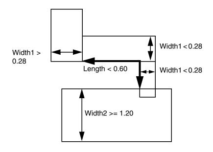
b) Violation; length < 0.60 is measured among all protrusion wires with width < 0.28.
