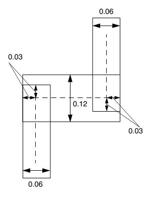
NDR1 has a width of 0.08 μm, so it will use the wrong-way width of 0.12, because 0.8 is less than or equal to 0.12 (the first wrong-direction width value). So a vertical route will have a width of 0.08 μm with extension of 0.04 μm on a vertical route, while a horizontal route will have a width of 0.12 μm with extension 0.04 μm:
