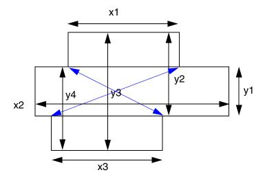
y1, y2, y3 & y4 should be checked against the given span lengths in SPANLENGTHTABLE without WRONGDIRECTION while x1, x2 & x3 should be checked against the span lengths in SPANLENGTHTABLE with WRONGDIRECTION. In addition, the length of the blue arrows should be checked against length.
