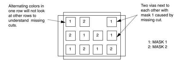
Unlike parameterized vias, there is no real row/column structure required in a fixed via, so the automatic coloring will not work well for a fixed via with missing cuts (or cuts that are not aligned). This type of via must be pre-colored to be useful.
