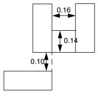
c) Okay. No overlap with notch above; therefore only default spacing of 0.10 required.
