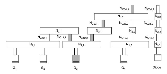
The router calculates the CAR with respect to gate G<sub>3</sub> after the cut C34 process step as follows:
