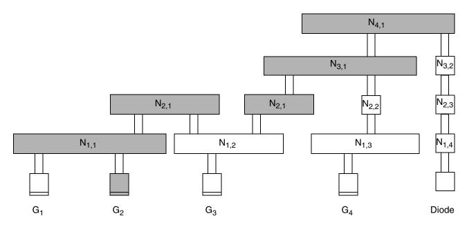
The path of the current between gate  $G_2$  and node  $N_{4,1}$  is shaded.
