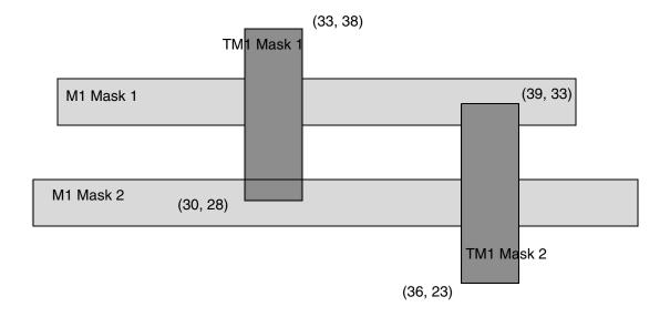
■ The following FILLS statement defines two rectangles and two via fill geometries for layer *metal1*. The rectangles and one of the via fill shapes require OPC correction.
