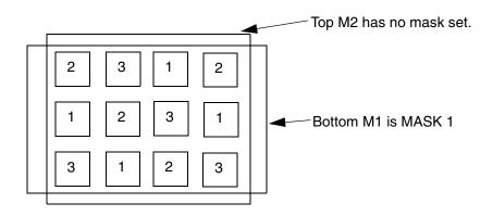
Masks for via-instance: ... ( 20 20 ) MASK 031 VIA1\_2 Bottom M1 is MASK 1.Top M2 has no mask set. Lower-left cut is MASK 3, and other via-instance cut shape masks are derived from via-master cut-masks as shown above by "shifting" the via-master masks to match: 1->3, 2->1, 3->2.
