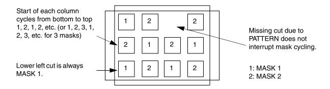
Assuming VIA1 is a 2-mask cut-layer, then the mask for each cut-shape is shown above. The default checker-board pattern is: the bottom left cut starts at 1, and goes left to right, 1, 2, 1, 2. The next row up starts at 2, and goes 2, 1, 2, 1, etc. Missing cuts due to PATTERN do not change the mask assignments.
