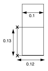
a) Violation. The 0.13 distance between the two convex corners marked with X is less than the wrong direction width of 0.2. It does not matter that 0.13 is larger or smaller than the 0.12 value in the other direction.
