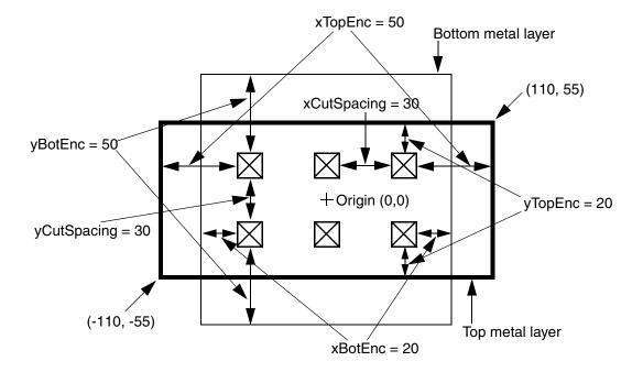
The same via rule with the following ORIGIN parameter shifts all of the metal and cut rectangles by 10 in the x direction, and by -10 in the y direction (see <u>Figure 4-26</u> on page 345):
