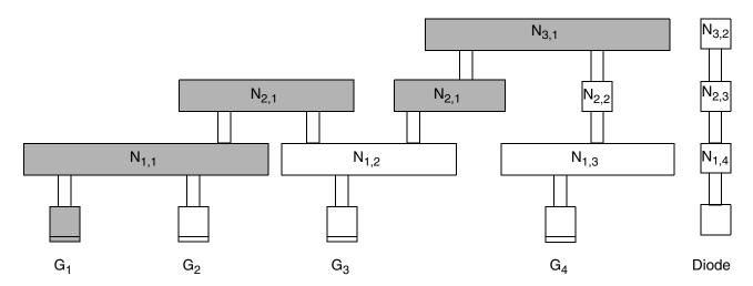
The path of the current between gate  $G_1$  and node  $N_{3,1}$  is shaded.
