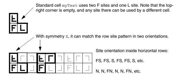
The following statement includes the gate-array site pattern syntax. It uses two F sites in a row with N (North) orientation.
