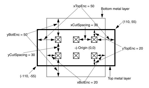
The same via rule with the following ORIGIN parameter shifts all of the metal and cut rectangles by 10 in the x direction, and by -10 in the y direction (see <u>Figure 1-50</u> on page 166):
