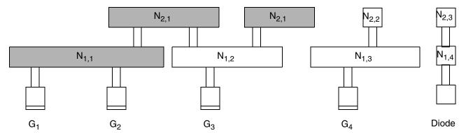
The path of the current between gate  $G_1$  and node  $N_{2,1}$  is shaded. Note that node  $N_{2,1}$  comprises two pieces of metal.
