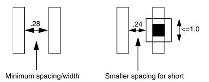
The USELENGTHTHRESHOLD argument specifies that the threshold spacing rule should be applied if the other object meets the previous LENGTHTHRESHOLD value.
