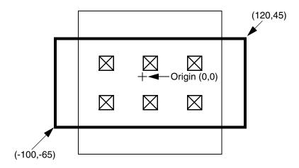
If the same via rule contains the following ORIGIN and OFFSET parameters, all of the rectangles shift by 10, -10. In addition, the top layer metal rectangle shifts by 20, -20, which means that the top metal shifts by a total of 30, -30.
