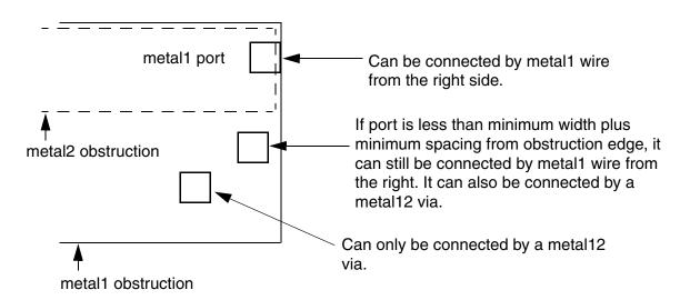
If a port is on the edge of the obstruction, a wire can be routed to the port without violations. Pins that are partially covered with obstructions or in apparent violation with nearby obstructions can limit routing options. Even though the violations are not real, the router assumes they are. In these cases, extend each obstruction to cover the pin. The router then accesses the pin as described above.
