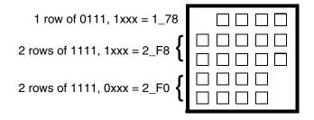
Figure 4-32 on page 351 illustrates the following via cut pattern syntax:
