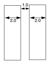
b) Okay if both wires are the same net and are either a power or ground net.
