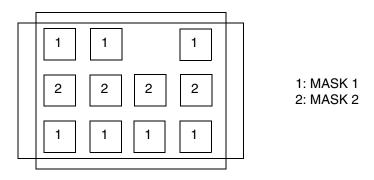
For a fixed via specified using RECT or POLYGON statements, the cut shapes must either be all colored or uncolored. If the cuts are not colored, they will be automatically colored in a checkerboard pattern as shown in <u>Figure 4-28</u> on page 346. Each via cut with the same lower-left Y value is considered as one row, and each via in one row is a new column. For common "array" style vias with no missing cuts, this coloring is a good one. For vias that do
