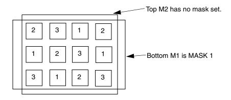
Masks for via-instance: + VIA VIA1 MASK 031 ( 0 25 ) Bottom M1 is MASK 1.Top M2 has no mask set. Lower-left cut is MASK 3, and other via-instance cut shape masks are derived from via-master cut-masks as shown above by "shifting" the via-master masks to match: 1->3, 2->1, 3->2.
