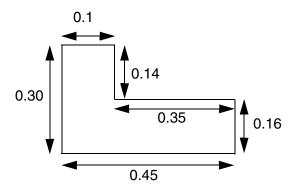
c) Violation, the 0.16 vertical segment would fail the wrong direction width requirement of 0.2.
