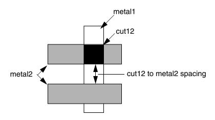
The "SPACING 0.15 LAYER metal2;" rule only applies to outside edges; therefore, no violations between cut12 and the top metal2 shape will occur. Only the spacing to the bottom metal2 shape is checked.
