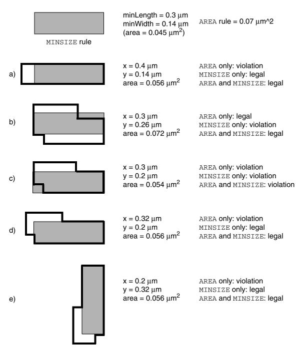
The following statement defines a MINSIZE rule that specifies that every polygon must have a minimum area of 0.07  $\mu$ m<sup>2</sup>, or that a rectangle of 0.14 x 0.30  $\mu$ m must be able to fit within the polygon, or that a rectangle of 0.16 x 0.26  $\mu$ m must be able to fit within the polygon:
