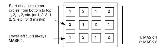
Uncolored fixed vias (from RECT/POLYGON statements) will get similar coloring as a parameterized via. Each cut with the same Y value is one row. The cuts inside one row alternate. This works well for cut-arrays without missing cuts as shown here.
