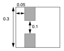
f) Okay. Extra cut is <= 0.2 away; therefore use min-width rule, and both cuts meet the min-width enclosure rule of 0.0 0.05.
