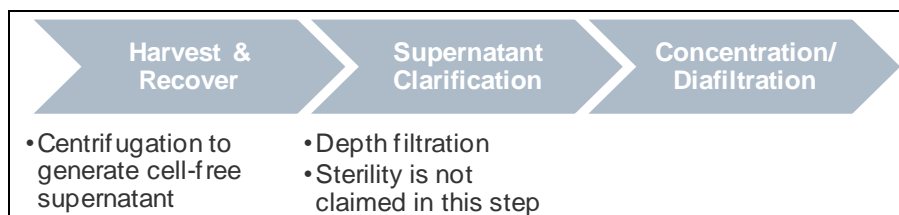
Figure 35. Clarification and concentration process flow.
