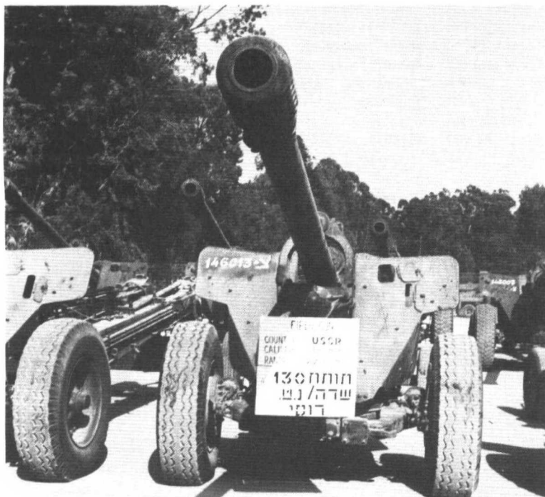
The Soviet 130mm field gun was used by the PLO for shelling northern Israeli settlements. The range of 2700 meters allowed the PLO to fire from behind UNIFIL positions in Lebanon and strike Israel.
