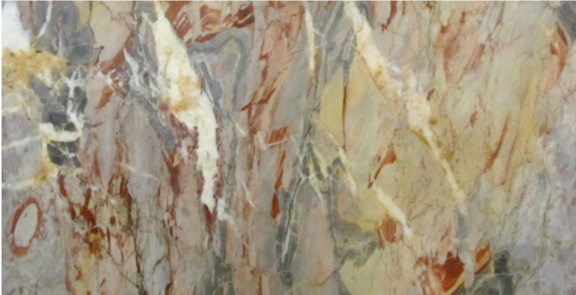
Sarrancolin Marble on the dining room walls, showing brecciation and fissures infilled with red and pink sediment, subsequently tectonised and cross cut by calcite-infilled tension fractures.
