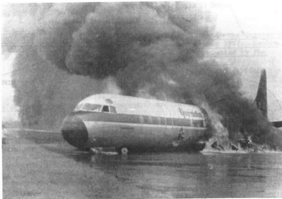
Figure 8-1. PK-GLB fuselage at standstill 225° heading, left wing separated. Spilled fuel burned fiercely. Note fuselage damage by No. 2 propeller.
