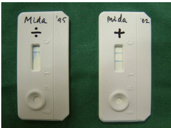
Fig. 1: RT test plates showing a negative and a positive reading
