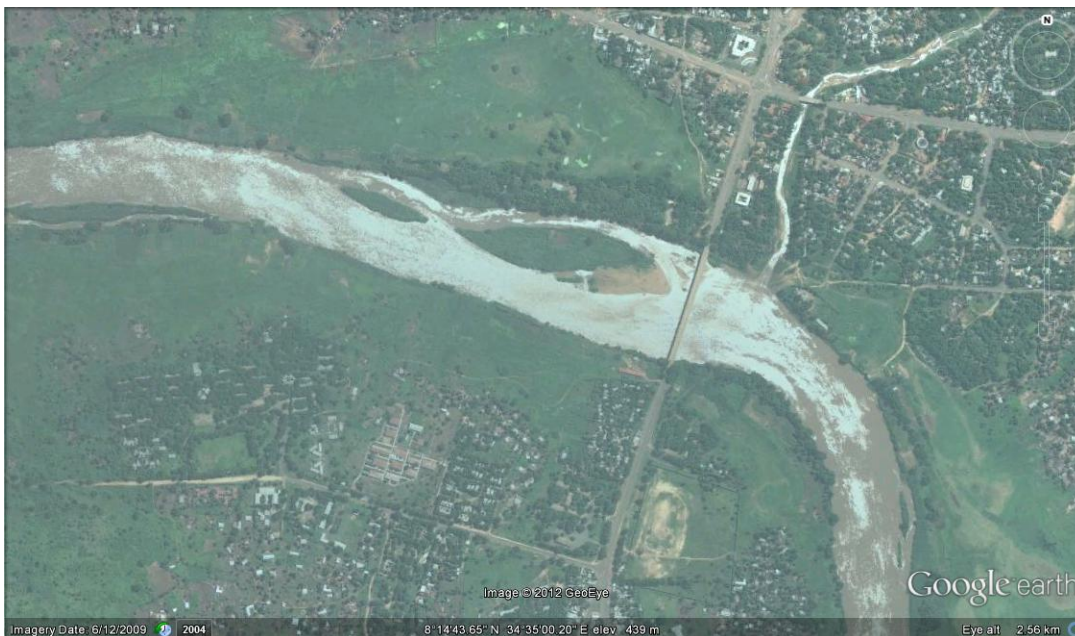
Figure 6.2 Gambela gauging station on Baro: discharge measured at bridge site and water level gauged 1 km downstream of bridge
