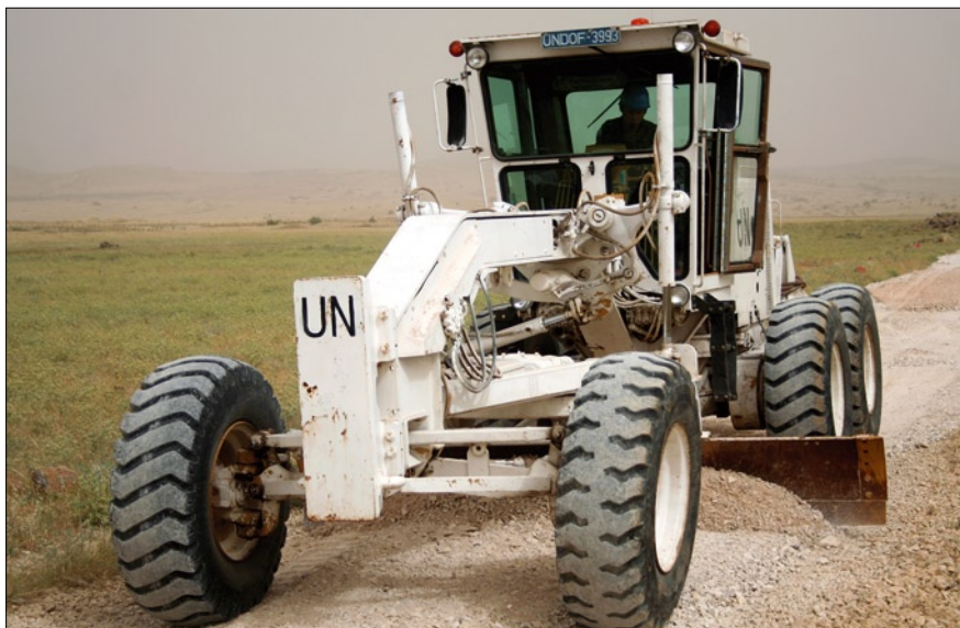
Grader maintaining a road
