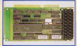
■ This is where the miracle happens. The large chip is the 68000 processor, below are two TOS 2.06 ROMs and along the right edge are the two SIMMs RAMs.
