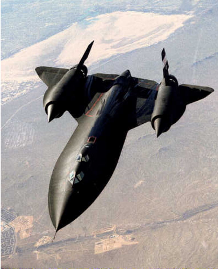
Figure 2 The high engine temperatures in the SR-71 Blackbird required a lubricant having extraordinary thermal stability. A polyphenyl ether was selected. [Photo courtesy NASA].
