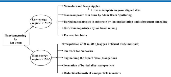
Fig. 1. Different possibilities of synthesis and engineering of the nanostructures by ion beam in low energy and high energy regime.
