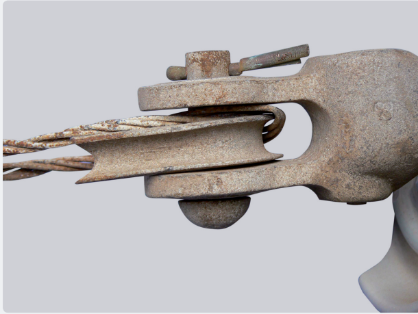
Figure 5.2 A jammed helical termination
