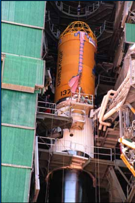
On Launch Pad 36-A at Cape Canaveral Air Force Station, a Centaur upper stage is mated to the lower stage Atlas IIA rocket for the GOES satellite launch.
