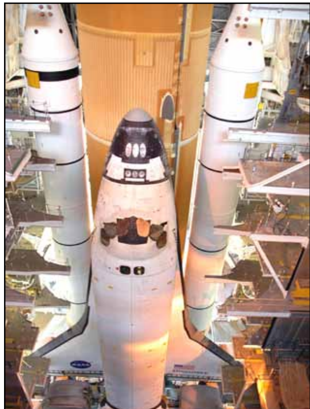
The elements of space shuttle Discovery are integrated in one of the cavernous high bays of the Vehicle Assembly Building. The platforms slide in and out, allowing workers to reach all levels of the vehicle. The shuttle is in the foreground and behind it is the huge external fuel tank, bracketed by solid rocket boosters.
