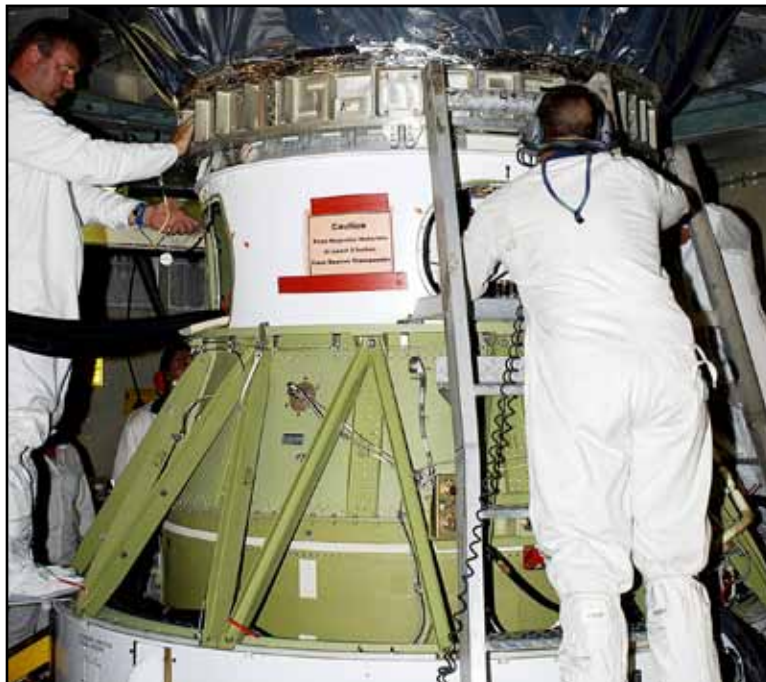
Workers on Launch Pad 17-B at Cape Canaveral Air Force Station, mate the Mars Exploration Rover Opportunity, to its Delta rocket. The second of twin rovers sent to Mars, Opportunity is equipped with a robotic arm, a drilling tool, three spectrometers, and four pairs of cameras that allow it to have a humanlike, 3-D view of the terrain. The rovers landed safely on Mars in 2004 and lasted much longer than their scheduled three-month mission.
