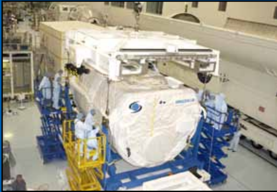
Payloads that will be carried into orbit by the space shuttle, such as the SHI Research Double Module (SHI/RDM), also known as SPACEHAB, are assembled and checked out in specially designed and equipped facilities at the spaceport.
