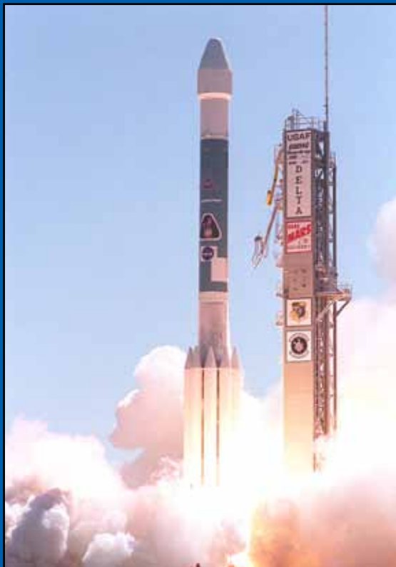
A Delta rocket lifts off from Cape Canaveral's Launch Complex-17 on April 7, 2001. The workhorse of the nation's space program, Delta has put into orbit more scientific, weather and communications satellites than all other vehicles of its class combined.
