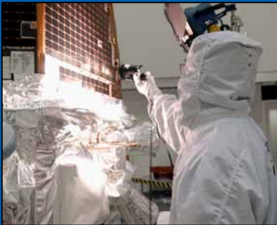
A worker conducts a light sensor test on NASA's Kepler spacecraft, set to survey the Milky Way galaxy for Earth-size and smaller planets in or near the habitable zone and determine how many of the billions of stars have such planets.
