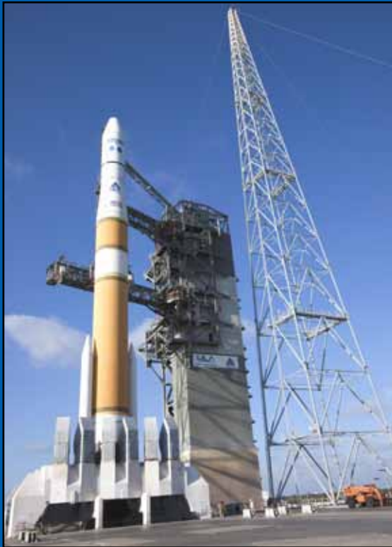
A Delta IV rocket awaits liftoff on March 4, 2010, on a flight to lift a weather satellite into orbit. Workers moved the mobile service tower back from the rocket on launch day to permit a launch. A satellite, called GOES-P, is inside the payload fairing at the top of the Delta IV.
