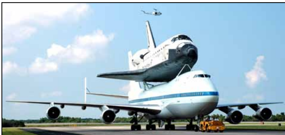
Space Shuttle Discovery, atop a modified Boeing 747 Shuttle Carrier Aircraft, is towed to the mate/demate device at the spaceport's Shuttle Landing Facility. The cross-country ferry flight became necessary when two days of unfavorable weather conditions forced Discovery and its STS-114 crew to land at Edwards Air Force Base in California.
