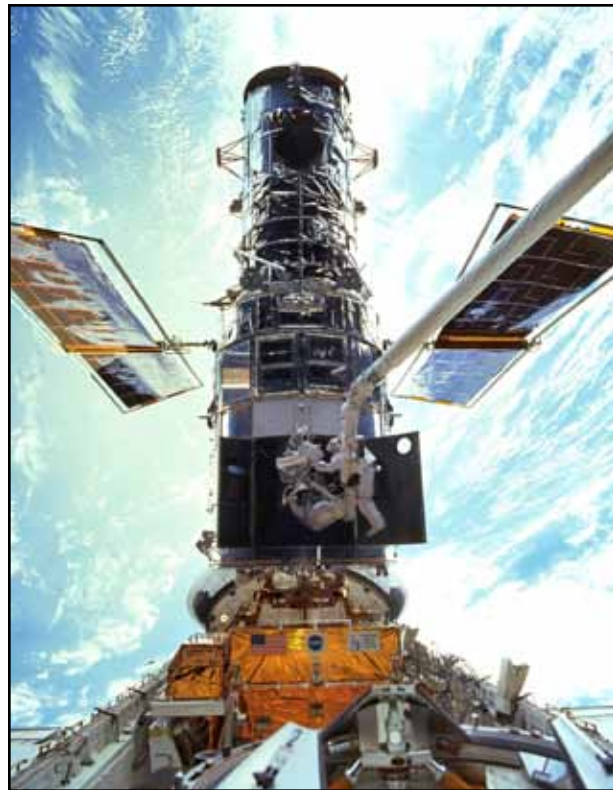
Astronauts Steven Smith and John Grunsfeld replace gyroscopes inside NASA's Hubble Space Telescope on the STS-103 servicing mission in December 1999.
