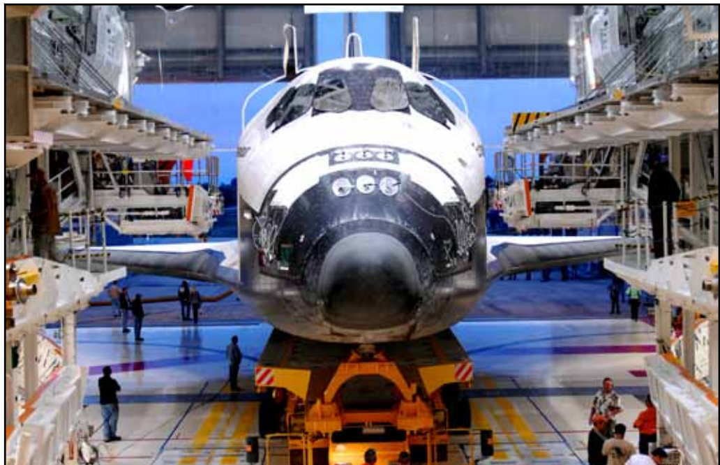
Space shuttle Endeavour begins backing out of Orbiter Processing Facility-2 for rolover to the Vehicle Assembly Building, where it will be mated with its external fuel tank and solid rocket boosters.
