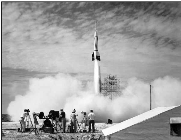
The modified German V-2 rocket takes off as the first launch from Cape Canaveral on July 24, 1950. The rocket attained an altitude of 10 miles. Note the primitive facilities, including a tarpaper shack serving as a blockhouse and the pad service structure made from painters scaffolding.
