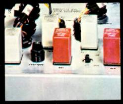
PELAYS MOUNTED ON CONTROL CENTER — The Wurfitzer 2800 introduces a convenient relay control center on the junction box which contains the selector circuitry and is controlled by five plug-in relays. These relays can now be checked as you would check vacuum tubes — a feature that saves time, speeds service and eliminates a goodly percentage of costly call-backs.
