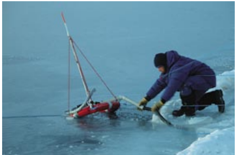
Launching a temperature probe into open water from the edge of the sea ice.
