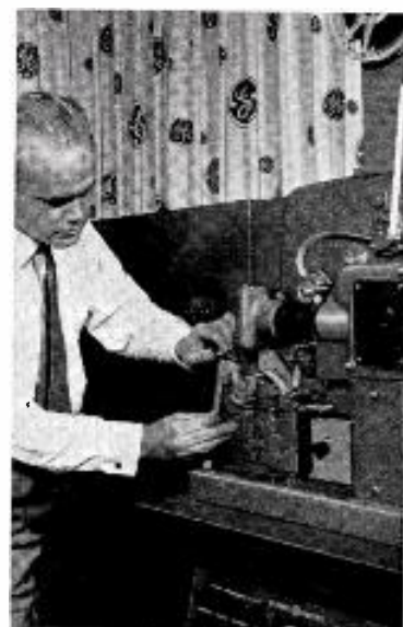
Film threading of the Eastman Continuous Motion 16 mm Projector is fast and easy. Light compensating mirrors, behind window, are out of the focal plane—eliminating dust problem—and rotate at 770 rpm.
