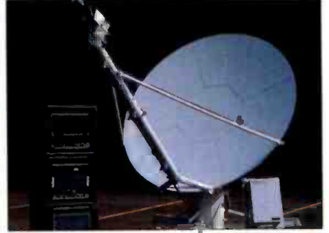
Harris's S-2D digital flyaway unit requires far less power (40 watts compared with 300) than do portable analog uplinks and can run off a DC battery in the field.
