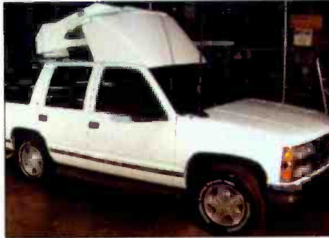
Harris's S-15 SNG vehicle puts a 1.2-meter microwave dish on a Chevy Tahoe body to achieve four-wheel-drive mobility.
