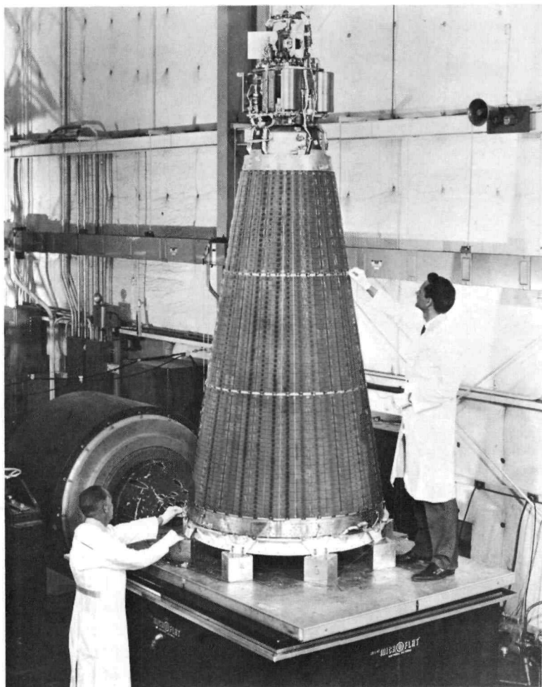
Figure 19 The complete SNAP-10A power plant showing the reactor perched on top of the conical radiator-thermoelectric element assembly (also shown on the cover). A rocket launch shroud surrounded this power plant during the launch period, but was blown off with explosive bolts once the reactor was in orbit.
