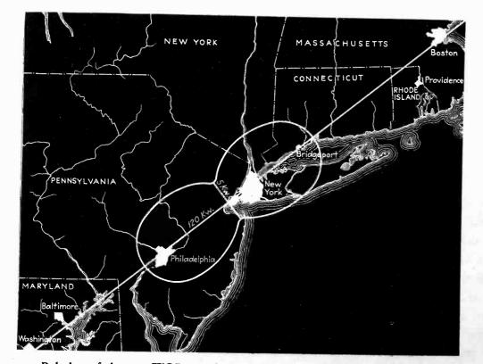
Relation of the new WOR signal to population. The hour-glass figure is the theoretical signal contour at one mile from the transmitting antenna, superimposed on the map of the service area. Note the amazingly large population centered on the axis of the 120 kw. signal
