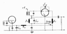
Delayed a.v.c. One plate of double diode is less negative than the other by the voltage across  $E_d$
