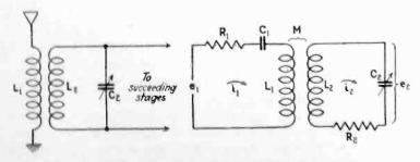
Fig. 1-Antenna and equivalent circuit
