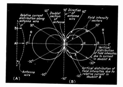
Fig. 1. (A) Typical vertical antenna, showing the current distribution and two doublets. (B) Field intensities radiated from doublets A and B at various angles above and below the horizon
