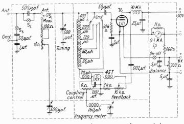
Fig. 2-Measuring set for antenna characteristics
