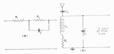
Fig. 4-Equivalent antenna circuit and (b) network to be used with antenna measurements
