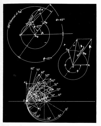
Fig. 7. Sample construction for the case of a vertical antenna operated at its third harmonic, described in text
