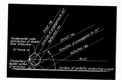
Fig. 2. A doublet located above a perfectly conducting ground. The reflections from the ground combine with the direct radiation, causing wave interference
