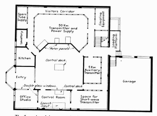
The floor plan of the transmitting building. The corridors surrounding the main transmitting equipment permits visitors to view it during operating hours
