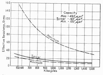
Fig. 3-Resistance characteritics of typical roof antennas
