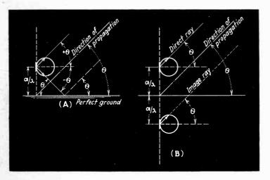
Fig. 3. In the diagram at the right, the effect of the ground reflections has been replaced by an "image doublet" located below the ground plane. The propogated waves in both cases are the same
