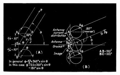
Fig. 4. (A) Doublet and image, expressed for the case of a doublet located one quarter wave above ground (cf. Fig. 5). (B) An antenna operated at its third harmonic, with current anti-nodes located at the ground and one half-wave length above it. (cf. Figs. 7 and 8.)
