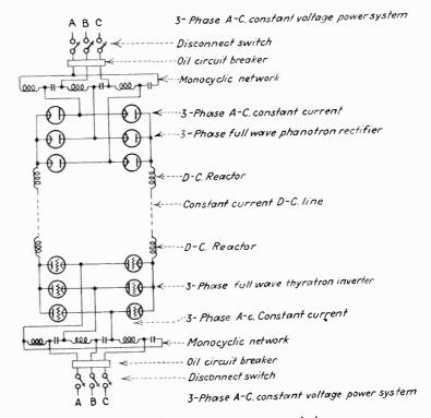
Block diagram of direct-current transmission system
