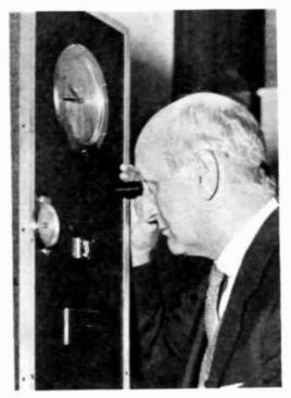
The crystal-oscillator electronic clock at the U. S. Naval Observatory now compares and sends its own broadcasts
