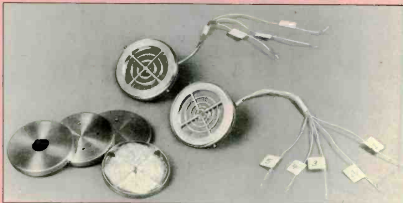
Bell's prototype four-bit (top) and six-bit (bottom right) digital transducers for telephones used all-acoustic "desampling" filters (pieces at bottom left).
