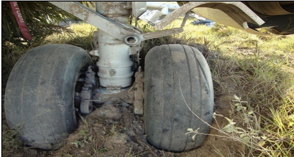
Figure 8: A Dirt Berm Marked the Final Resting Position of the Main Gear Tires
