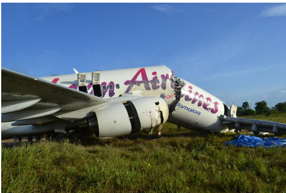
Figure 11: Showing break in first class cabin, deployed R1 slide, and open right over wing emergency exits and partially extended thrust reverser door
