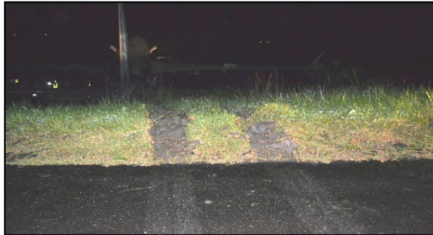
Figure 7: Under carriage tire marks off the runway.
