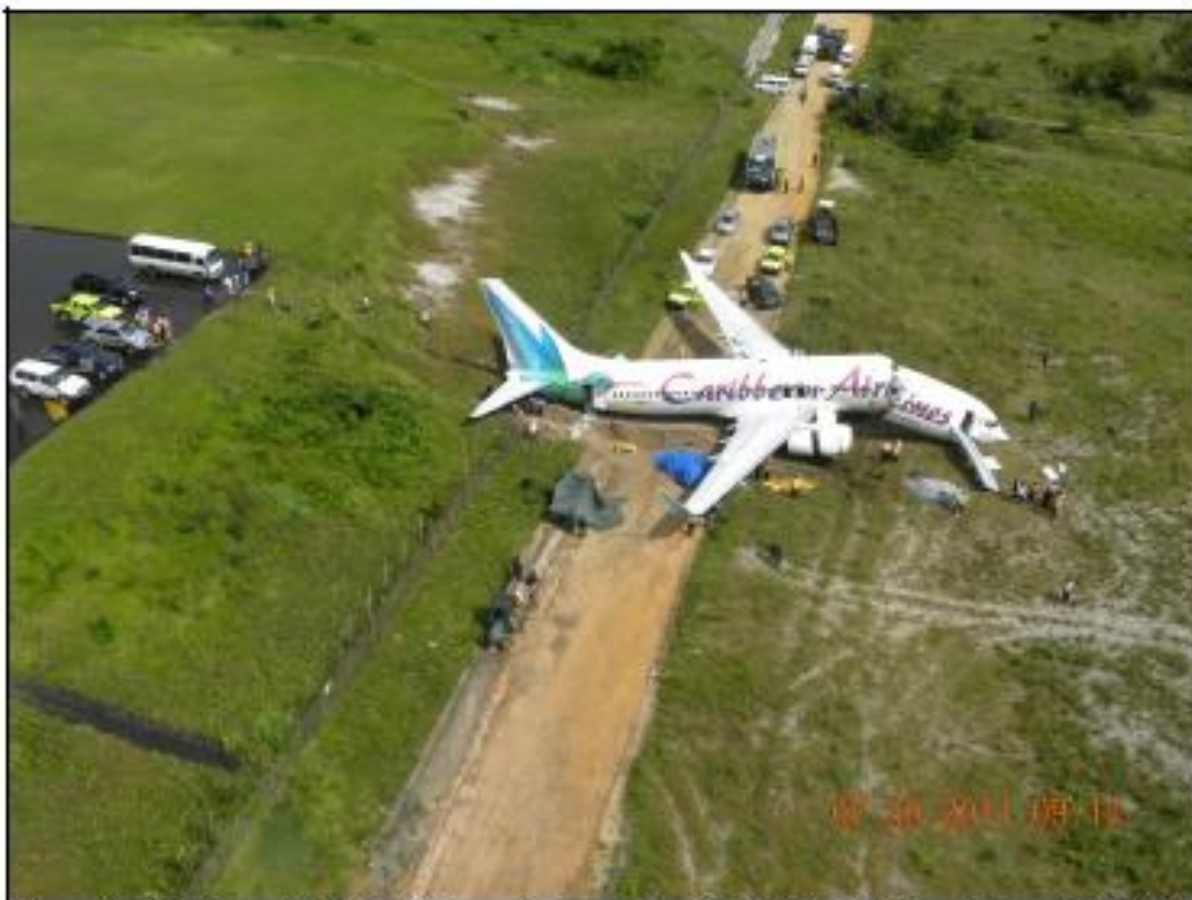
Figure 3: Caribbean flight 523 Stopped Approximately 130 ft Off of the End and 64 ft Left
