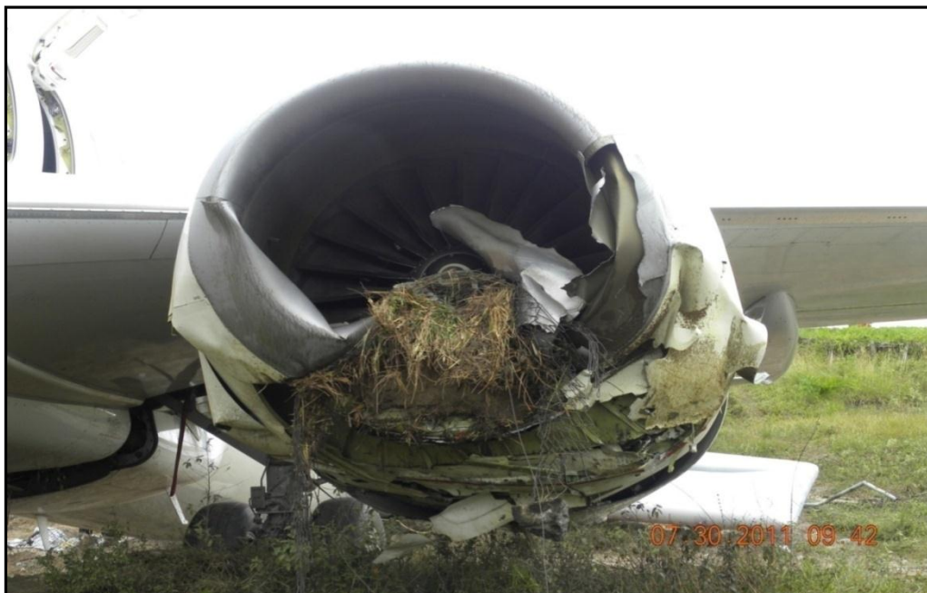
Figure 12: Mud and Grass were found on Both Nacelles
