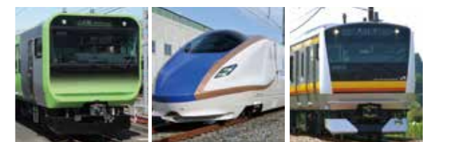
E235 series: The Yamanote line was equipped with a state-of-the-art train information management system E7 series: The Hokuriku Shinkansen that incorporates the highest level of cutting-edge technology E233 series: VVVF inverter cars for commuter and suburban transportation
