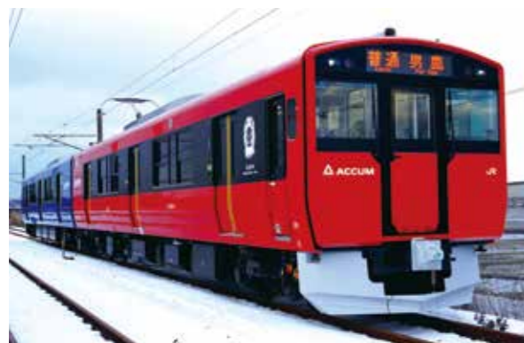
EV-E801 series Accumulator railcar train for use on alternating current (AC) section
