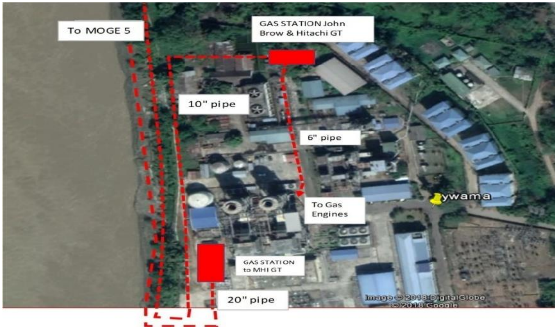
Figure 3-5: Gas Pipelines in the Plant Area
