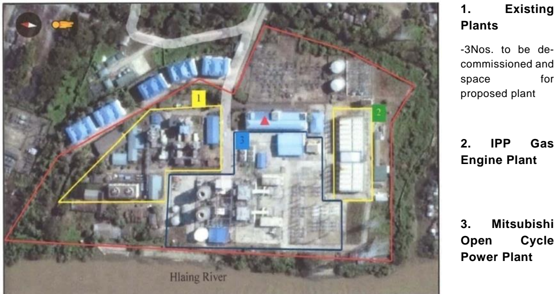
Figure 1-1: Existing Plant Layout
