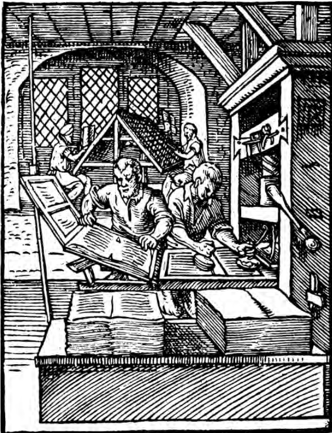
Early wooden printing press, depicted in 1568. Such presses could produce up to 240 impressions per hour.
