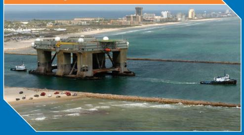
The Heavy Lift Device, capable of lifting more than 13,000 tons, raises the huge radar in Kiewit Offshore Services at Ingleside, Texas.
