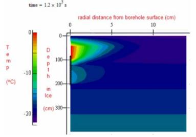
**FIGURE 8**: Thermal model results at 20 minutes indicating further melting near the piezoelectric stack but no melting at the bit/ice interface.
