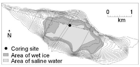
Figure 4: Bathymetric map of Lake Vida based on GPR and ice coring. GPR transect lines are shown. Solid black circle is the coring site.
