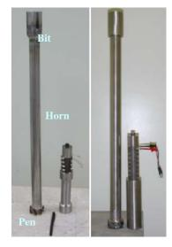
**FIGURE 9**: A view of the solid and dog-bone shape actuators next to the U/S Gopher coring bits.
