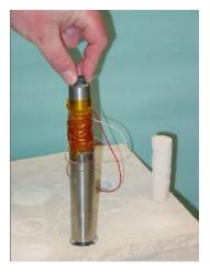
**FIGURE 3**: A photographic view of a prototype Ultrasonic/Sonic Gopher that drilled limestone and the core that was created.
