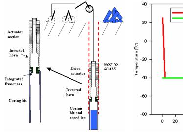
**FIGURE 6**: Schematic view of the ultrasonic-gopher operating inside the borehole.
