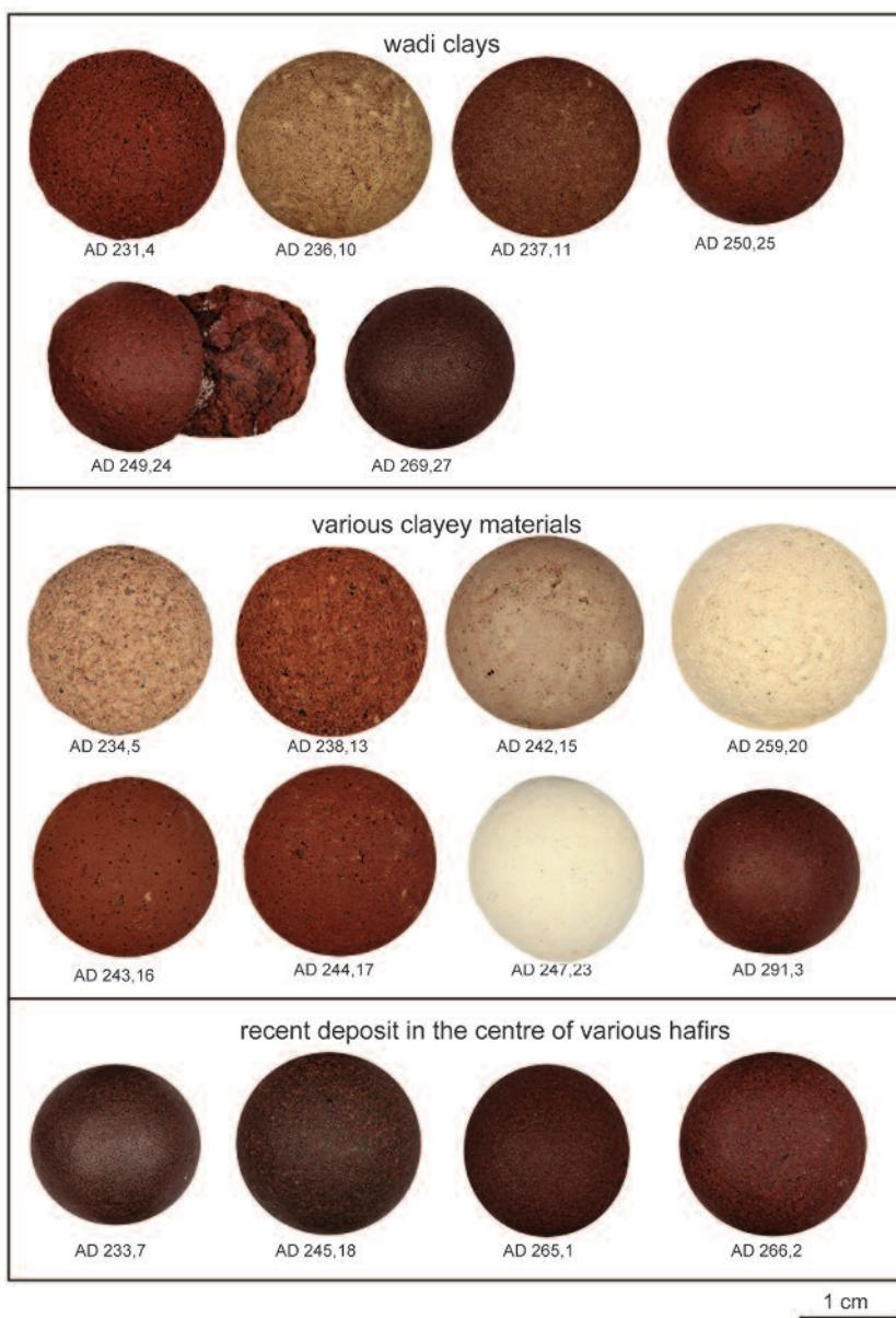
Fig. 16. Specimens of various raw materials fired at 1200°C
