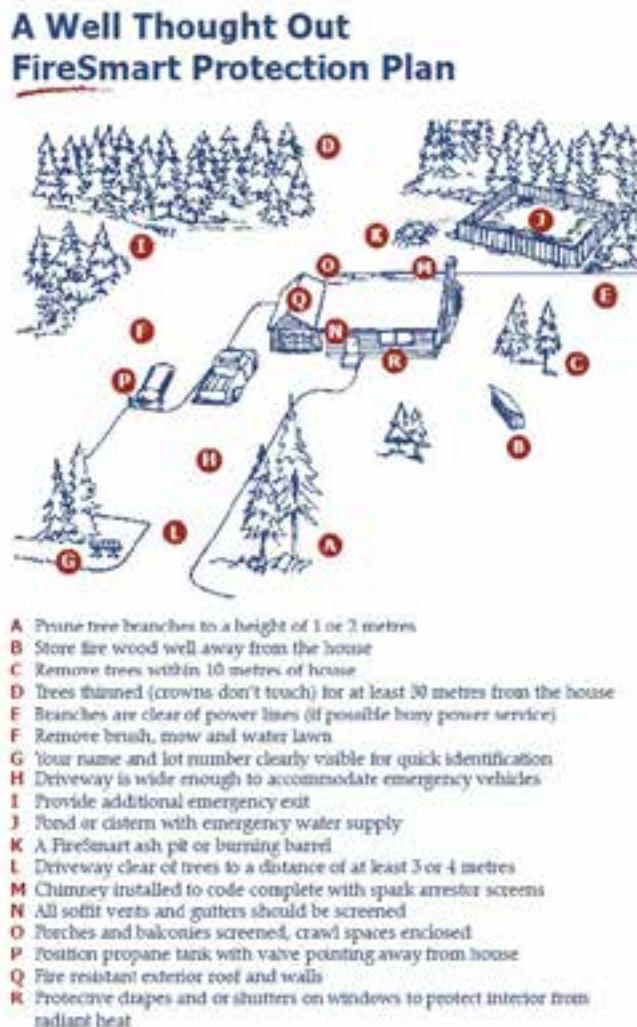
Figure 11. Illustration of a FireSmart Protection Plan for a private home from The Homeowners FireSmart Manual. Source: Ontario Government and Partners in Protection.
