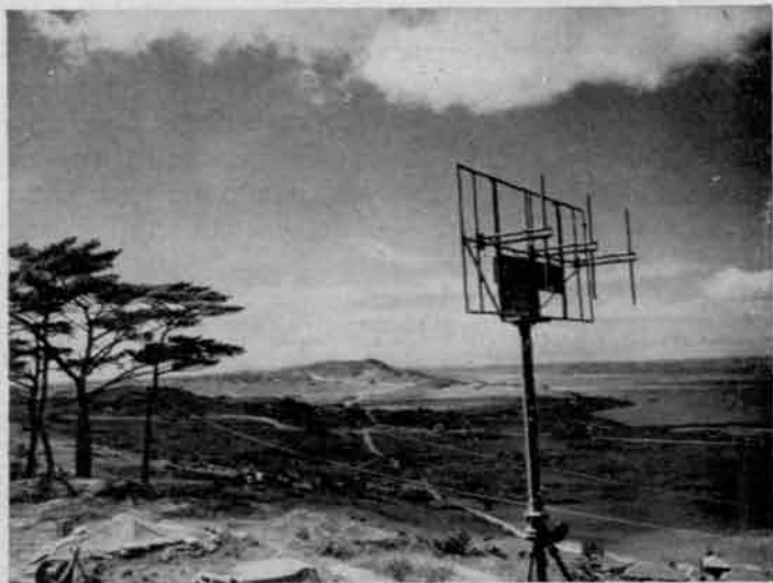
IFF Antennae of Hqs. Btry 504th AAA Gun Bn overlooking Buckner Bay
