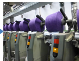
Open-end spinning => recycled yarn
