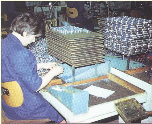
Assembly of hose clamps at Wattholma Bruk 1967–68
