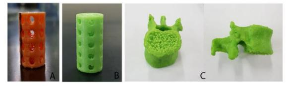
FIGURE 7. 3D prints. (A) NaCl template with 4 holes. (B) NaCl template with 5 holes. (C) Vertebrae bone.
