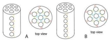
FIGURE 1. NaCl template for material research apparatus. (A) Design 4 holes. (B) Design 5 holes.
