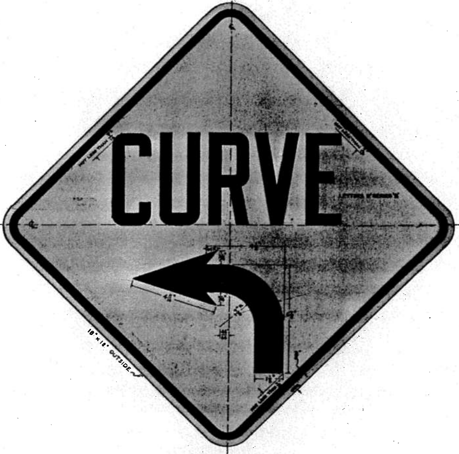
Figure 5: Slow Sign—Curve Letters, symbols and border, solid black Background, federal yellow (See Recommendation 21)
