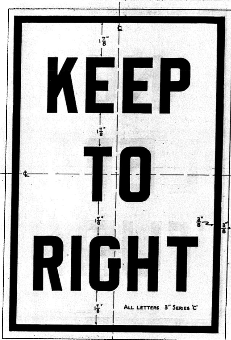
18" x 18" OUTSIDE Figure 9.: Information Sign—Keep to Right Letters and border, solid black Background, white (See Recommendations 31, 32, 34)
