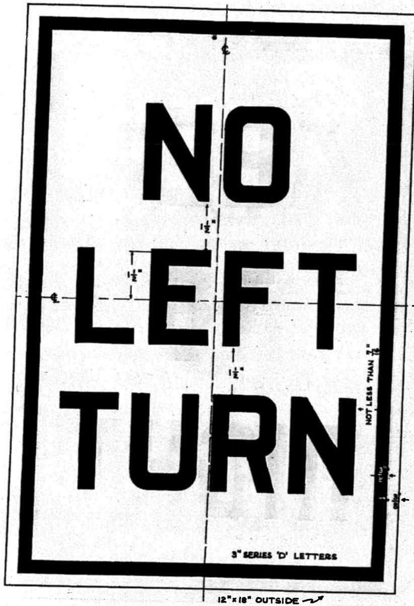
Figure 10: Information Sign—No Turn Letters and border, solid black Background, white (See Recommendation 33)
