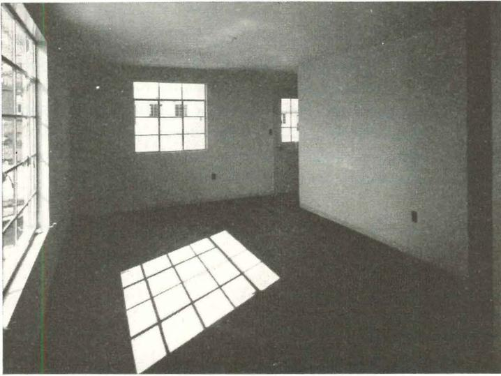
**THIS SMALL ROOM LOOKS SMALL** because its walls and partitions are cut up arbitrarily with window and door openings of different sizes and different heights. Low window and door heads produce dark splotches on ceiling; middle-of-the-wall fenestration leaves the corners of the room dark.
