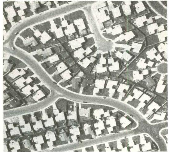
**DO** use curves, loops, cul-de-sacs to slow traffic, create visual variety. Use long blocks (up to 2,000') to reduce intersections, save on paving, utilities.
