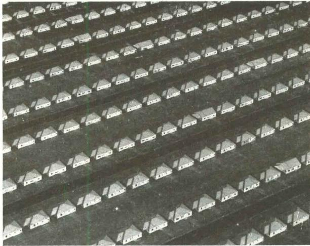
**DO NOT** lay out streets on a grid; it encourages through traffic, speeding, accidents at four-way intersections. Street scenes are endlessly drab and monotonous.
