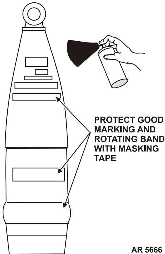
Figure 3-20. Using Spray Paint for Touchup.
