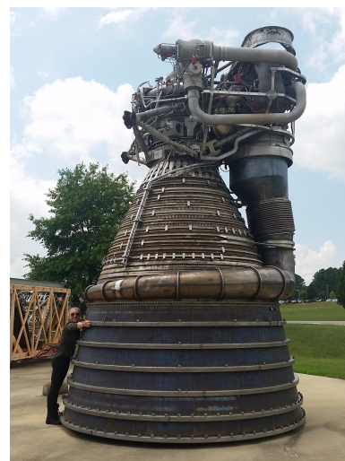
Figure 3: The F-1 rocket engine was used on the Saturn V launch vehicle that sent astronauts to the Moon. The large bell-shaped portion of the engine is called the nozzle . Notice the human (me!) in the photo for size scale. The first stage of the Saturn V used five of these engines!
