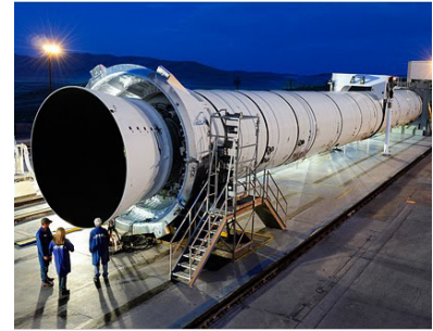
Figure 10: Solid rocket booster for the Space Launch System (SLS). The entire length of the booster, except for the nozzle, is filled with solid propellant. This is the largest solid rocket booster ever tested!
