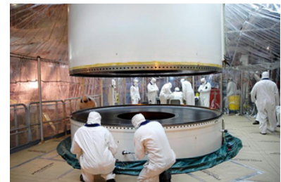
Figure 9: Two segments of the solid rocket booster for the Space Shuttle are being fitted together in this photo. The boosters are constructed out of four segments in total. It's easier to produce smaller segments of the solid propellant and assemble them together rather than make one big segment of solid propellant. Notice that the solid propellant has a hole in the middle.
