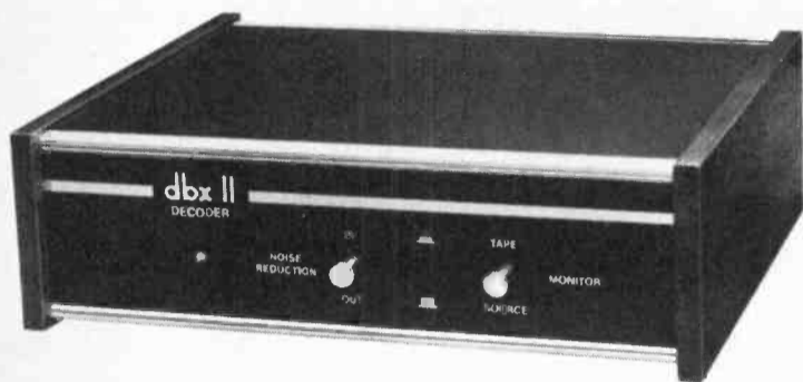
Audiophile Add-On: The basic dbx 21 disk decoder is used for decoding dbx-encoded disks as well as dbx digitally mastered full dynamic range recordings.
