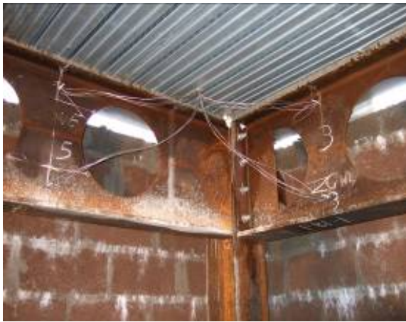
Figure 8-24 : TC locations for atmosphere temperature
