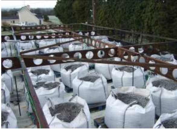
Figure 8–27 : a) Vertical static load b) Wooden cribs used for the fire load
