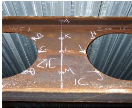
Figure 8-24 : TC locations for atmosphere temperature
