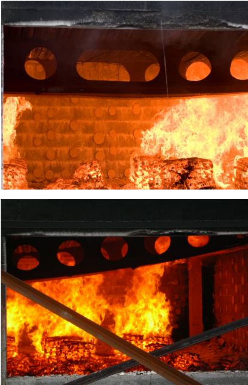
Figure 8–38 : Deflection of Long cellular beams in real fire
