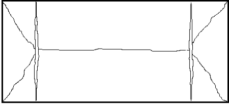
a- Crack forming at the intersection of the yield lines
