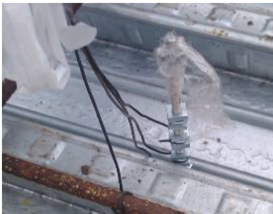
Figure 8-25 : Positioning of Thermo couples
