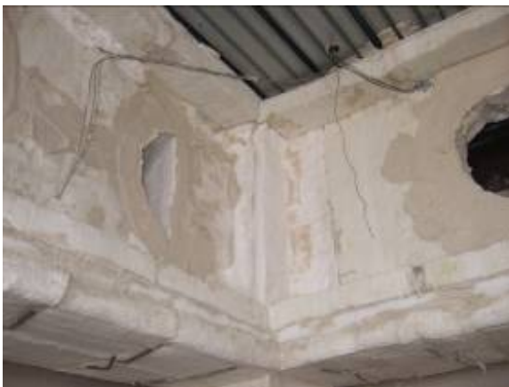
Figure 8-25 : Positioning of Thermo couples
