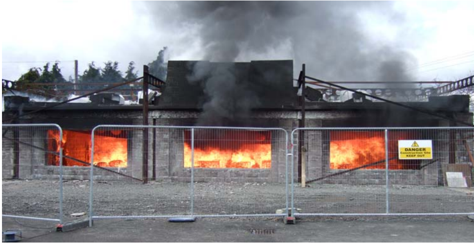
Figure 0–11 : Compartment in fire test.
