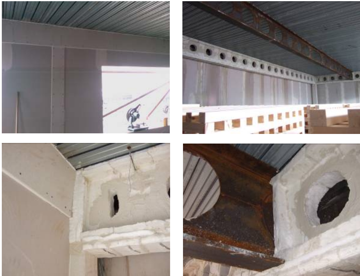
Figure 8–14 : Board and fiber protection used inside the compartment
