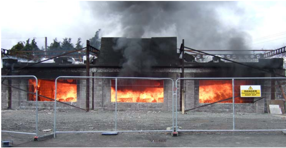
Figure 10–3 : Compartment in fire test.
