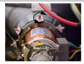
FIGURE 7. Geometry adjustment magnets (five visible; eight total)
