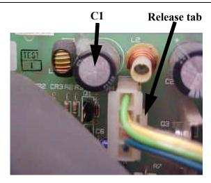
To disengage the connector, squeeze on the release tab and pull the top half out from the bottom half. Needlenose pliers are helpful here. The connector may be difficult to loosen, so don't be surprised if you have to struggle a little bit. Just be patient and work carefully and gently. If you rush, you run the risk of a sudden release, and you might hurt yourself (or the Mac) if you strike something.
