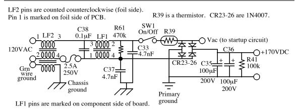
The switching power supply proper has three different subparts. One is a feedback controller, another is the actual switching converter, and the final is an array of output rectifiers and filters. The latter two subcircuits are where the most frequent failures occur.
