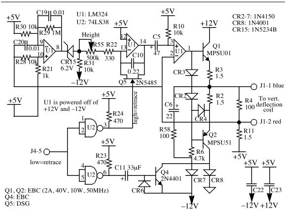
FIGURE 11. Vertical sweep generator
