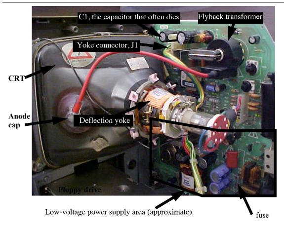
Some of the components you may be working with are identified in the photo. One is the yoke connector (the yoke gets its name from the fact that it sits around the neck of the CRT, just as a conventional yoke sits on the necks of oxen). Many common problems are caused by a bad yoke connector and/or its solder joints.
