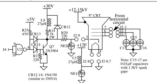
IC U2 is a quad open-collector NAND, one gate of which is connected as a simple inverter to present the video signal to Q7 with the proper polarity (a low at J4-1 corresponds to white). Resistor R25 is the NAND gate's pullup resistor. Diodes CR13 and CR14 form a "Baker clamp" to prevent saturation of Q7 when driven hard, thereby speeding up response.
