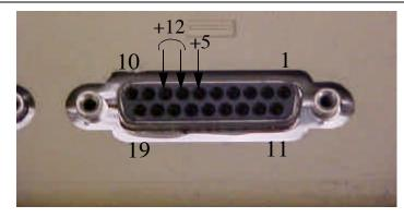
Adjust the +5V line to 5.00V, then verify that the +12V line hasn't been forced too far from +12 (it should be below 12.75V, and above 11.9V). It's probably not a bad idea to make these measurements both cold and hot, to make sure that there's no thermal drift to speak of.
