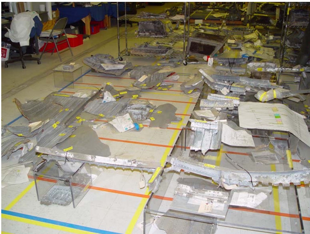
Figure 2.4-40. Lower forward fuselage skin and frame debris.
