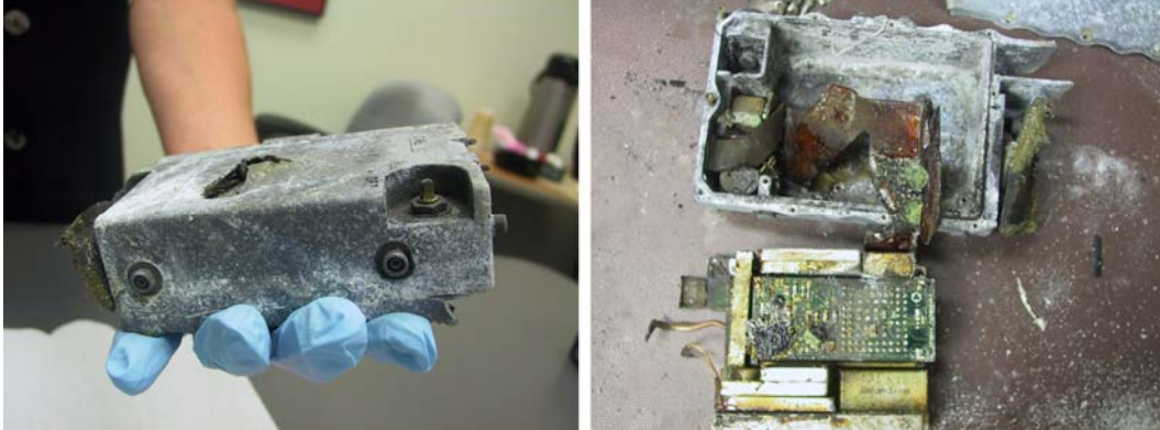
Figure 3.2-33. External (left) and internal (right) views of a recovered Army/Navy personal radio communications-112 radio.
