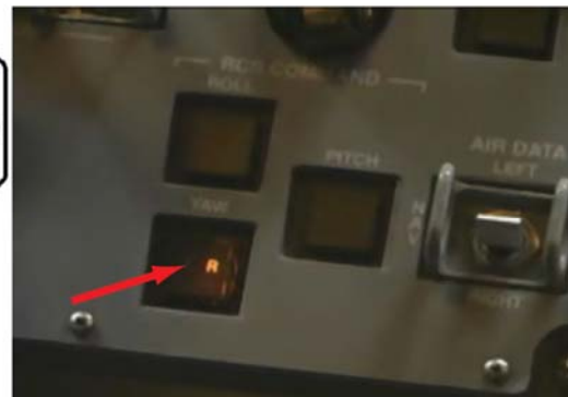
Figure 1.2-37. Reaction Control System thruster status display. [Pictures [top and bottom left) adapted from the Space Shuttle Systems Handbook; picture (bottom right) from the Shuttle Engineering Simulator]
