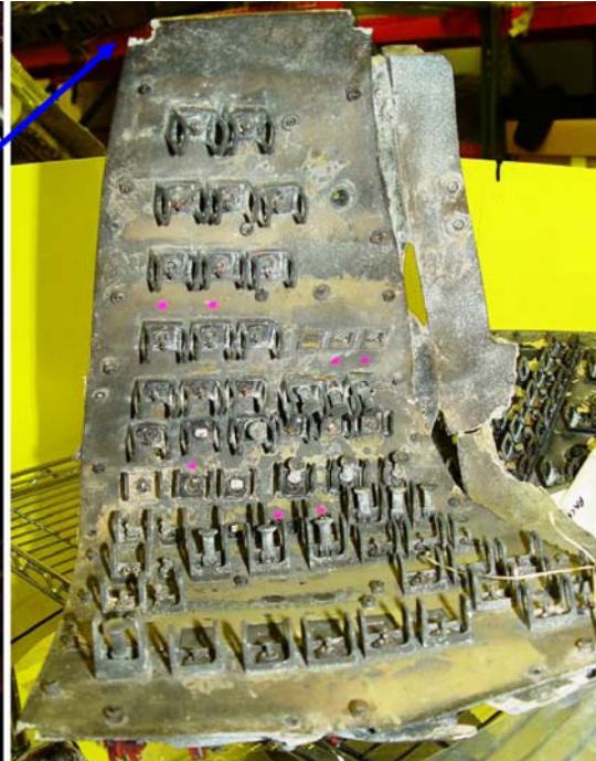
Figure 3.4-11. Recovered R2 panel from Columbia (after it was unfolded). Pink dots are above the out-of-configuration switches.
