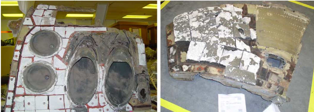
Figure 2.4-24. Two large forward Reaction Control System debris pieces, Columbia Reconstruction Database debris item nos. 792 (left) and 82061 (right).
