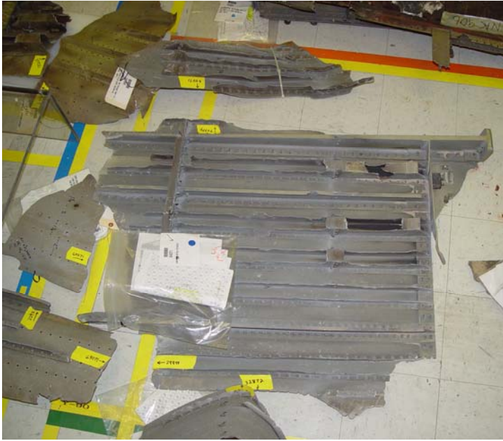
Figure 2.4-41. Lower forward fuselage skin panel near external tank attachment.
