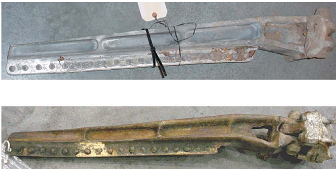
Figure 1.1-25. Port x-link, debris item no. 1678 (top), and starboard x-link, debris item no. 1765 (bottom), from the Columbia Reconstruction Database.
