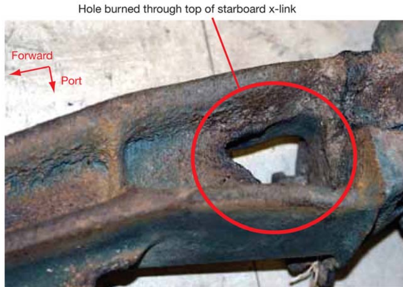
Figure 2.1-49. Close-up of the hole in the starboard x-link. [Columbia Reconstruction Database, debris item no. 1765]
