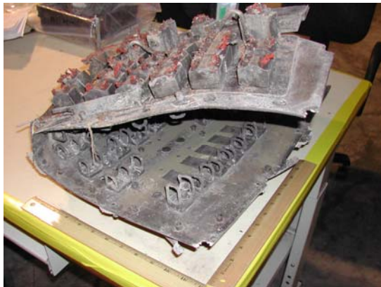
Figure 3.3-3. Recovered R2 panel from Columbia.
