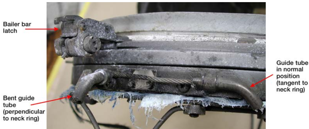
Figure 3.2-24. Hold-down cable guide tube.
