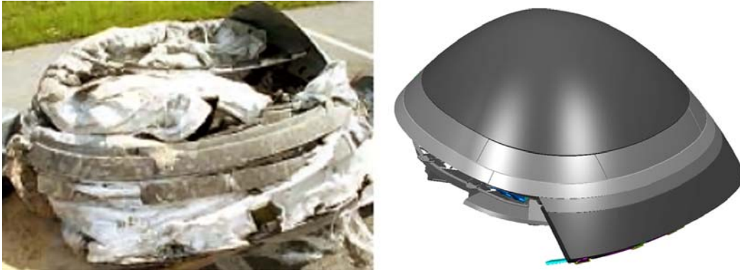
Figure 2.4-23. Nose cap Columbia Reconstruction Database debris item no. 1114 vs. the original nose cap with chin panel.
