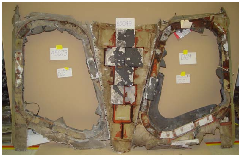
Figure 2.4-38. Forward fuselage arrowhead panel and the forward two windows, facing in.
