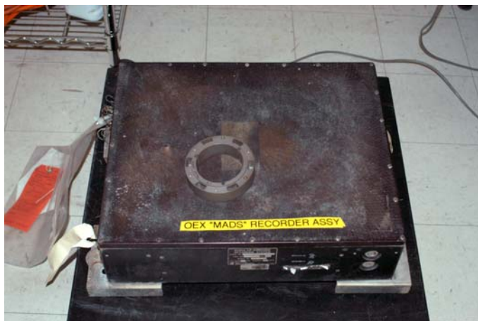
Figure 2.1-44. Recovered orbiter experiment recorder from STS-107. [Columbia Reconstruction Database, debris item no. 54057]
