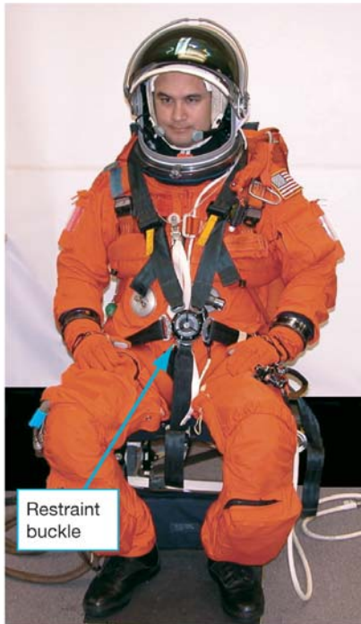
Figure 3.1-39. Demonstration of the five-point seatbelt buckle.
