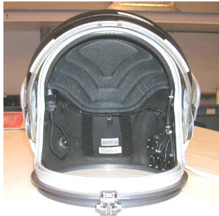
Figure 3.4-19. Example of an intact, pristine advanced crew escape suit nonconformal helmet (not an STS-107 helmet).
