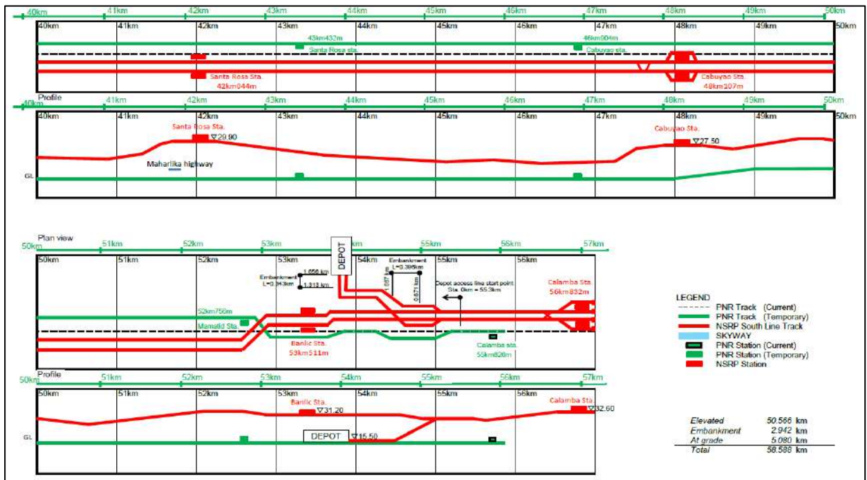
Figure 3.4.5 Outline diversion plan of exiting PNR tracks (3 of 3)
