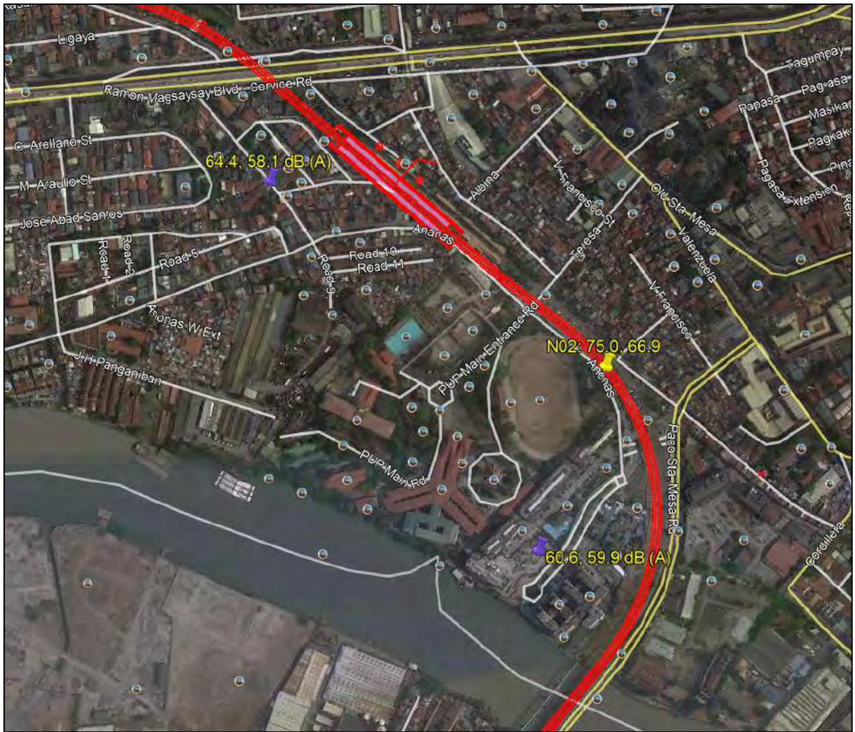
Figure 3.3.33 Locations and Noise Level Measurements, Yellow Pin N02 for 2018 Wet Season and 2019 Dry Season Periods while Purple Pins are the Additional Noise Measurements conducted in Sept-Oct. 2019. Note the Drop in Noise Levels with Respect to Distance from the Project Alignment and the Shielding Effect of Intervening Buildings.
