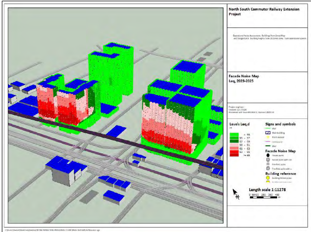
Figure 3.3.62 Façade Noise Map of the Cluster of Buildings at the Corner of Buendia and South Luzon Expressway Approaching the Buendia Station to the left
