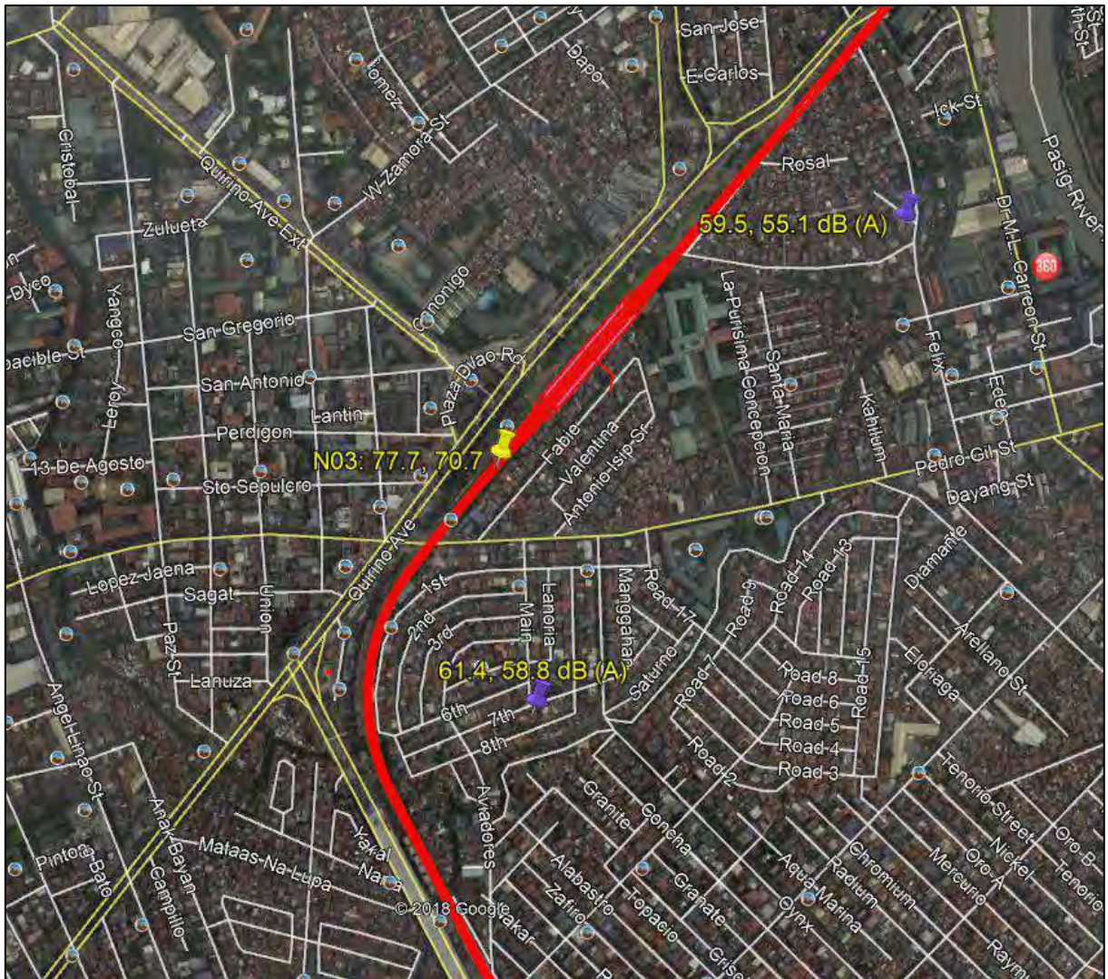
Figure 3.3.34 Locations and Noise Level Measurements, Yellow Pin N03 for 2018 Wet Season and 2019 Dry Season Periods while Purple Pins are the Additional Noise Measurements conducted in Sept-Oct. 2019. Note the Drop in Noise Levels with Respect to Distance and from the Project Alignment and the Shielding Effect of Intervening Buildings.
