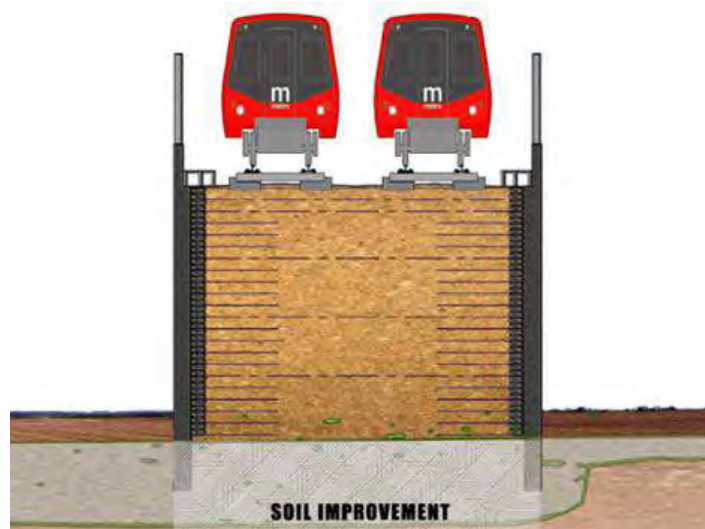
Figure 1.4.3 Cross-section of a typical embankment
