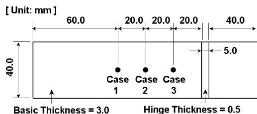
Fig. 2. Geometry of a strip part (mm) with a hinge and gate locations used in CAE analyses.
