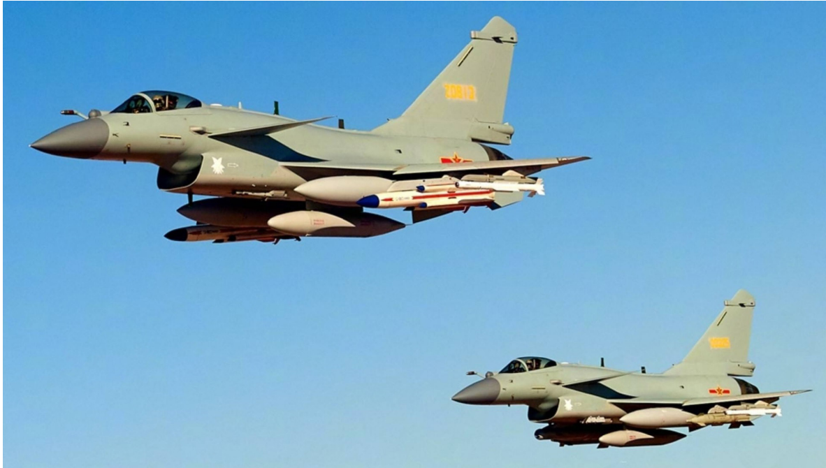
Figure 9: J-10Cs With Anti-Radiation Missiles, PL-10s and Laser-Guided Bombs
