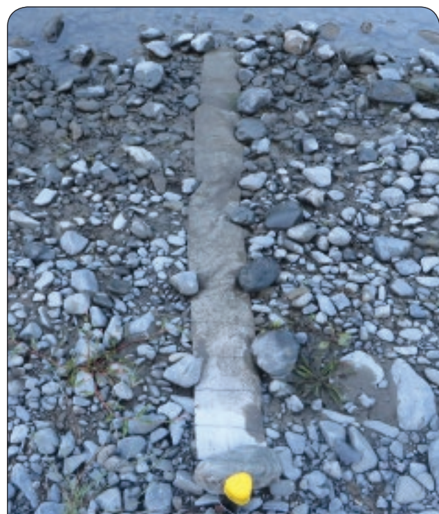
FIGURE 5 // Sediment deposition on geotech fabric placed on the banks of the Rangitikei River to record sediment deposition during the February and March flushes (Photo: Opus).
