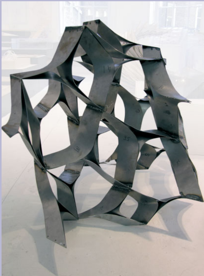
Production of a full-scale prototype. Left: Partial prototype. Right, top to bottom: Laser-cut steel strips, tangency alignment of strips, and spot welding of the aligned strips.
