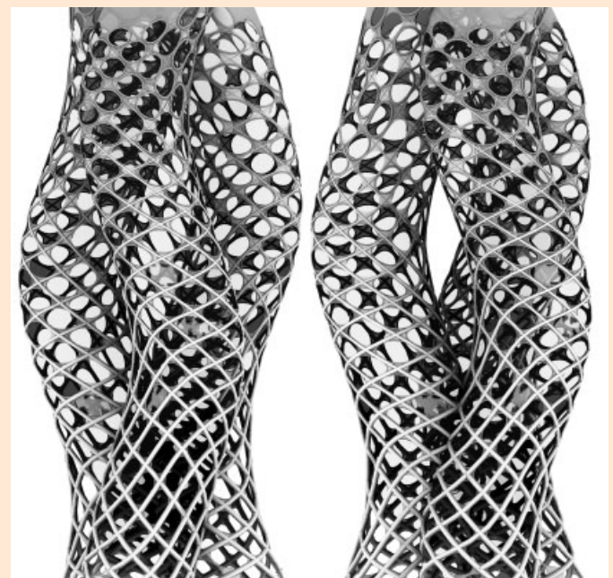
Digital image (two elevation views) of the structural skin developed as a bundled structure. A composite-based system combining the structural strands with additional surface members is articulated to create a structurally differentiated envelope in which force flows are distributed along its entire surface.
