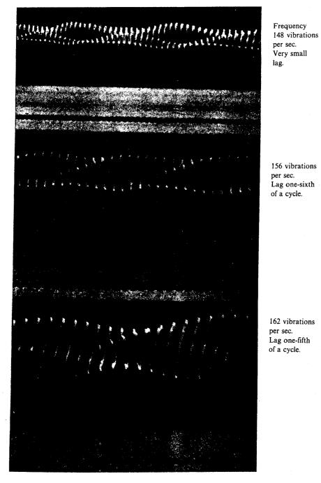
Plate XXV. Cyclical vibrations of G-string and bridge of 'cello near 'wolf-note' pitch, showing the differences in lag.
