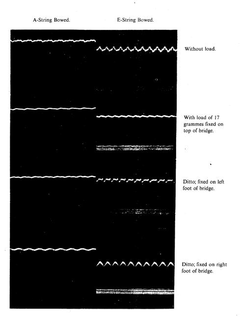
Plate VI. Simultaneous vibration-curves illustrating effect of loading the bridge on its horizontal motion transverse to the strings, (observed at the G-string corner).
