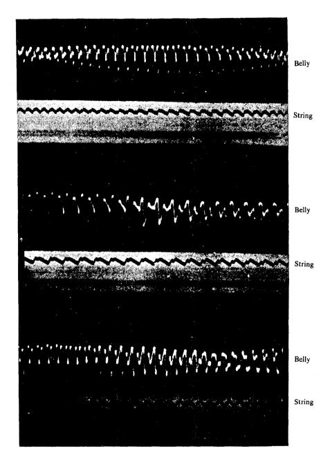
Plate II. Simultaneous vibration-curves of belly and G-string of violoncello at half the "wolf-note" pitch showing the resonance of the octave and cyclical changes.
