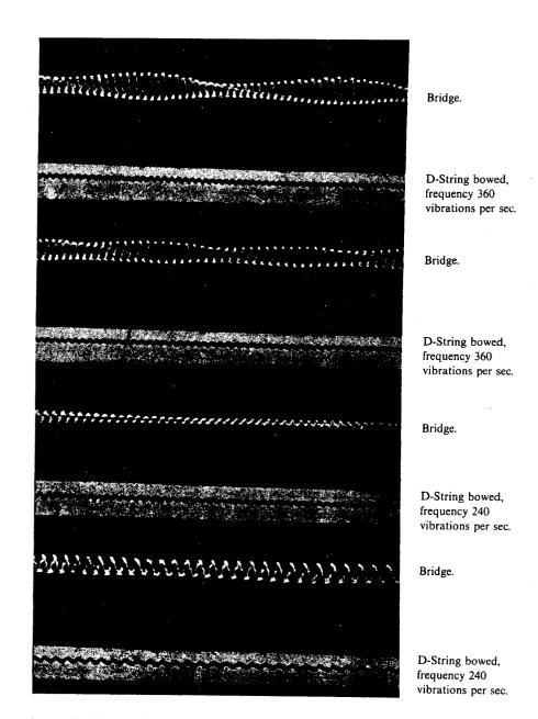
Plate X. Simultaneous vibration-curves of the bridge and D-string of a violoncello, showing cyclical changes at frequencies other than that of the "wolf-note".
