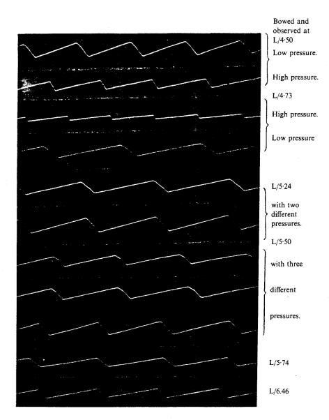
**Plate VIII.** Modified two-step zig-zag vibration-curves at the bowed point, showing the practical constancy of the velocity of ascent with the bow, and the variability of the velocity of descent against the bow.
