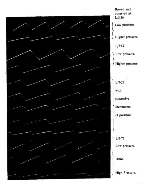
Plate VII. Modified two-step zig-zag vibration-curves at the bowed point, showing the practical constancy of the velocity of ascent with the bow, and the variability of the velocity of descent against the bow.
