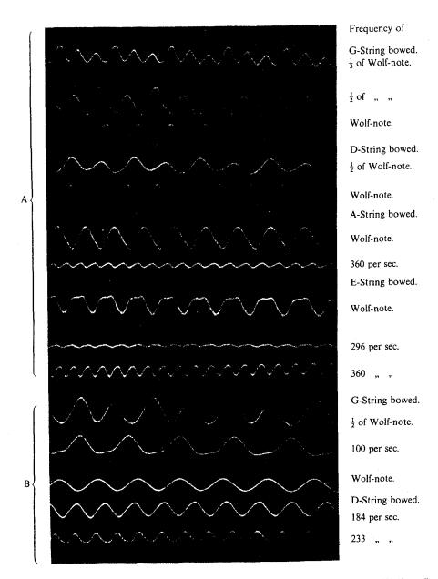
Plate IV. Resonance-curves of belly of violoncello. A. Without any load on the bridge: "Wolf-note" frequency 176 vibrations per second. B. With a load of 40.4 grammes fixed on top of bridge. "Wolf-note" frequency 137 vibrations per second.
