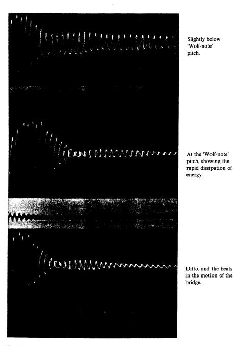
Plate XXIV. The simultaneous vibration-curves of the bridge and G-string of a 'cello (plucked).
