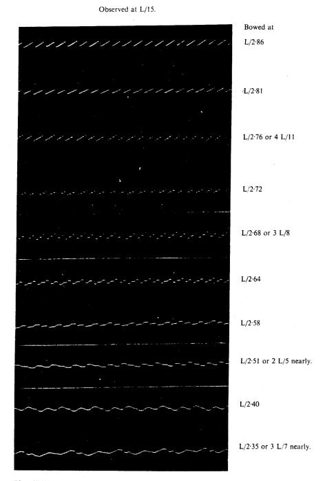
Plate XVII. The third (negative) type of vibration: its rational and transitional modifications.
