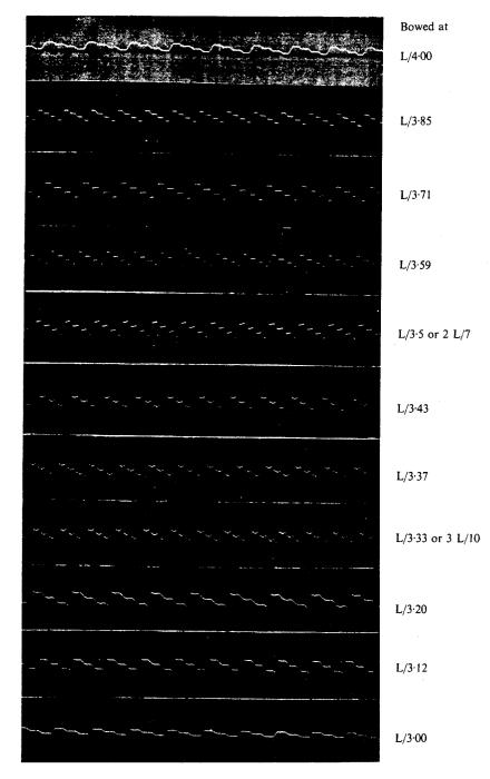
Plate XII. The first type of vibration: its rational and transitional modifications.
