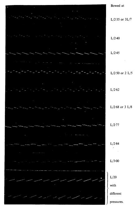
Plate XVI. The second type of vibration: its rational and transitional modifications.
