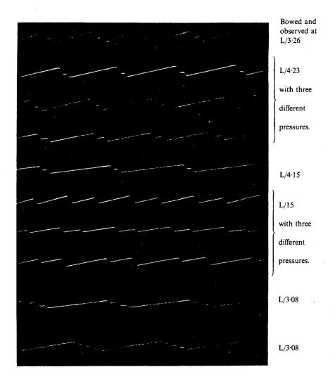
Plate IX. Modified four-, six-, and eight-step zig-zag vibration-curves at the bowed point, showing the practical constancy of the velocity of ascent with the bow, and the variability of the velocity of descent against the bow.
