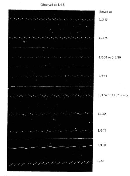
Plate XVIII. The third (positive) type of vibration: its rational and transitional modifications.
