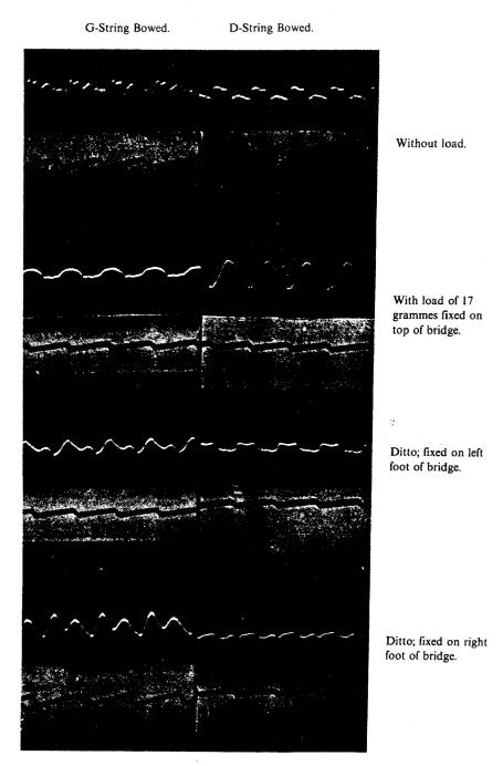
Plate V. Simultaneous vibration-curves illustrating effect of loading the violin bridge on its horizontal motion transverse to the strings (observed at the G-string corner).
