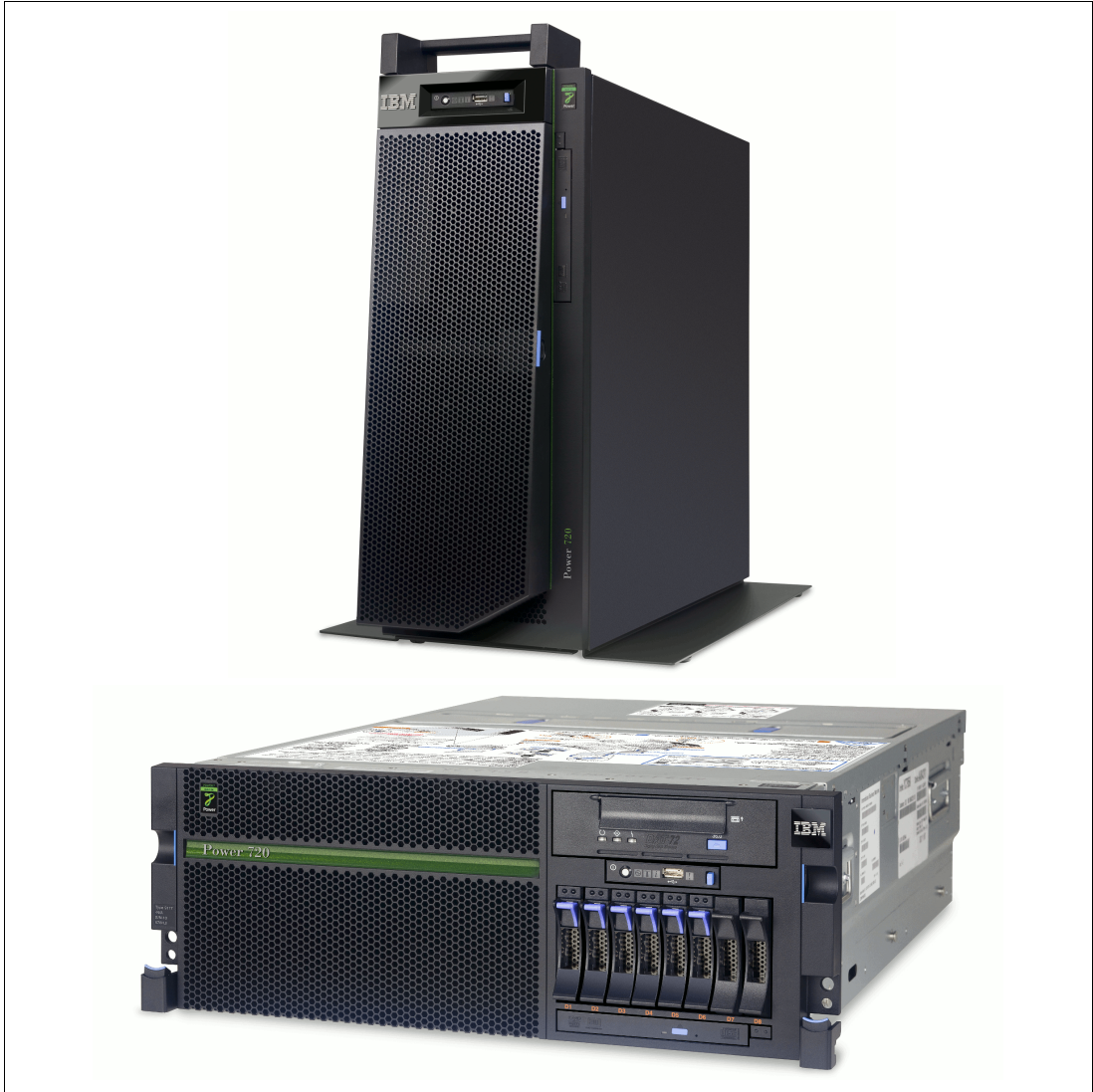
Figure 1-1 Power 720 rack and tower models
