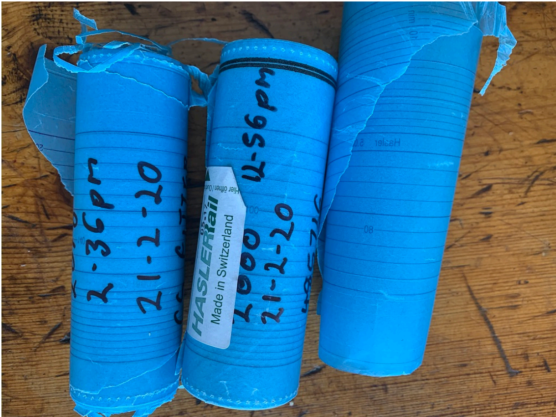
The photograph shows the recovered waxed tapes. The centre roll is the tape from power car XP2000. The left and right rolls are the tape from power car XP2018 that jammed and was torn at one location. Source: CITS
