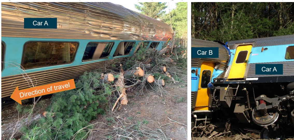
The left photograph shows Car A rolled to its left and supported by pine trees, and the right photograph shows the trailing end of Car A bound with the leading end of the next car, Car B. Source: CITS
